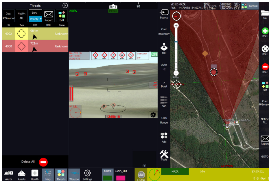
Fig. 9 Example of the robotic vehicle gunner WMI display. The left portion is the threats screen widget where the gunner can easily identify potential targets. The center portion is the sensor display. In the sensor display, the camera sensor data come from ARES. It shows where the weapon system is aimed. Additional features include the red boxes denoting ARES-identified targets, and the newly added target detection widget (oval at the bottom of the screen). The right portion of the WMI is the map widget, as depicted in Figs. 6–8.
