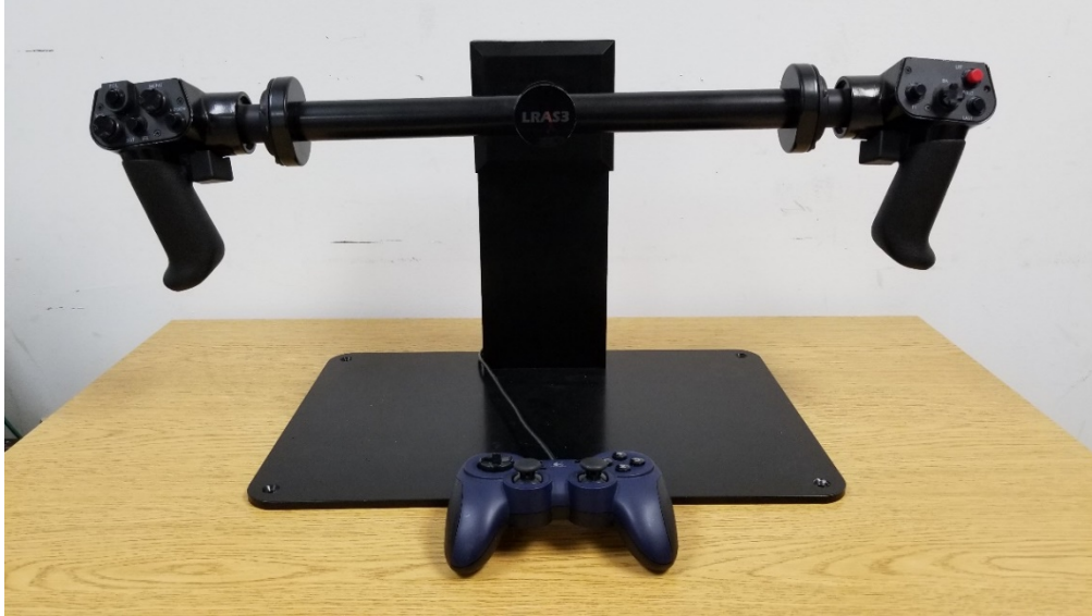
Fig. 3 LRAS3 handgrips (for control of the LRAS3) and gamepad (for control of operator's head movements) are used for integrating the LRAS3 operator crewstation into the Wingman SIL
