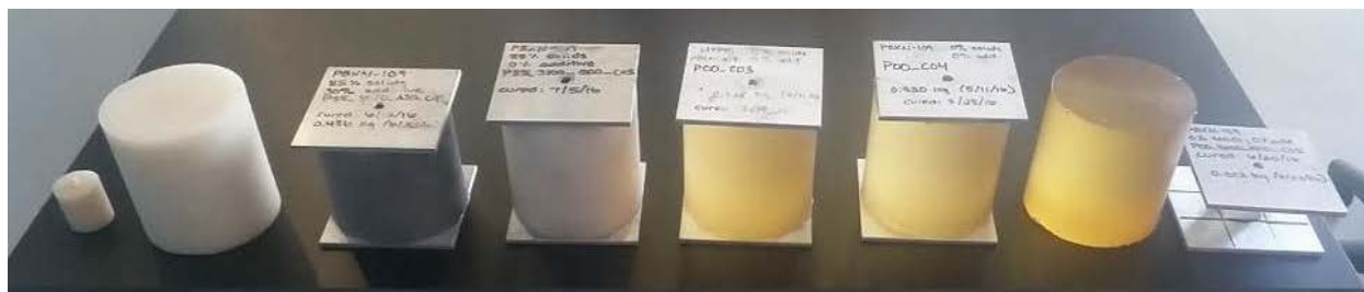
Figure 4. The different PBXN-109 formulated (mock) samples with different compositions and geometries that are subjected to sinusoidal and random base excitation testing
