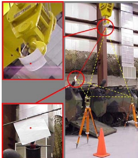
Figure 20 Typical BEAMS setup depicting the tetrahedron formed by theodolites and screens (Laser line and spots enhanced for clarity.)
