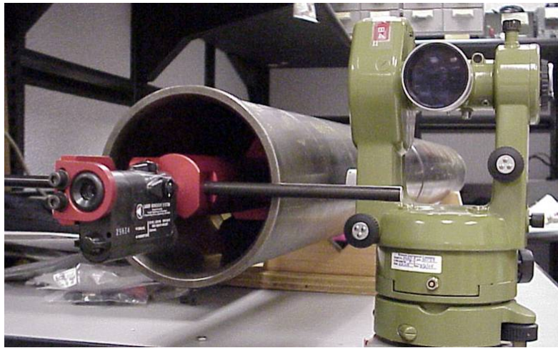
Figure 17 Theodolite placed adjacent to laser apparatus during calibration
