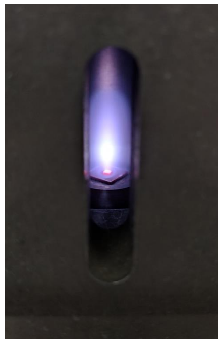
Growth of superconducting diamond in a highly dense CVD plasma
