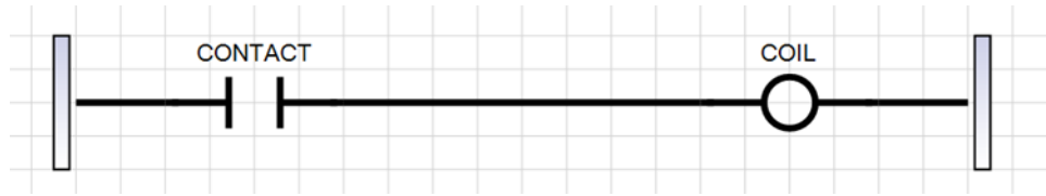
Figure 19. Ladder diagram rung inside function block diagram program.
