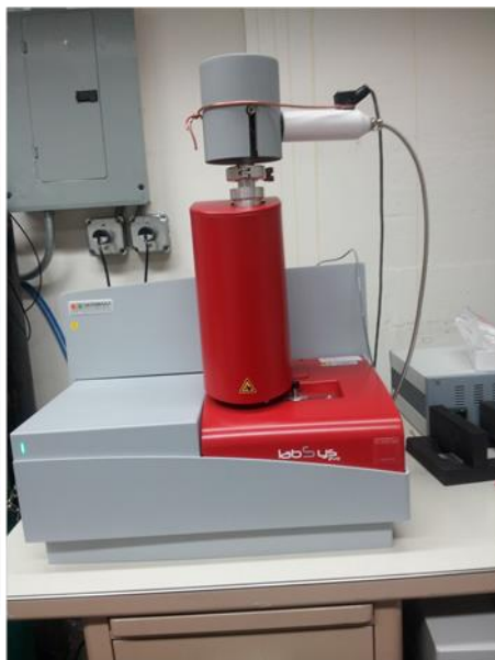
Figure 5. The TGA/DSC experimental system.
