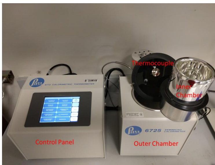
Figure 1. The bomb calorimeter for heat release measurements.
