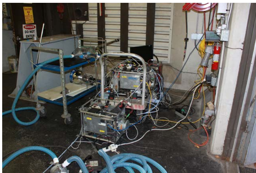
Fig. 36 A photo of the sampling and control electronics, and plumbing for sample extraction, exterior to the ARL small blast chamber
