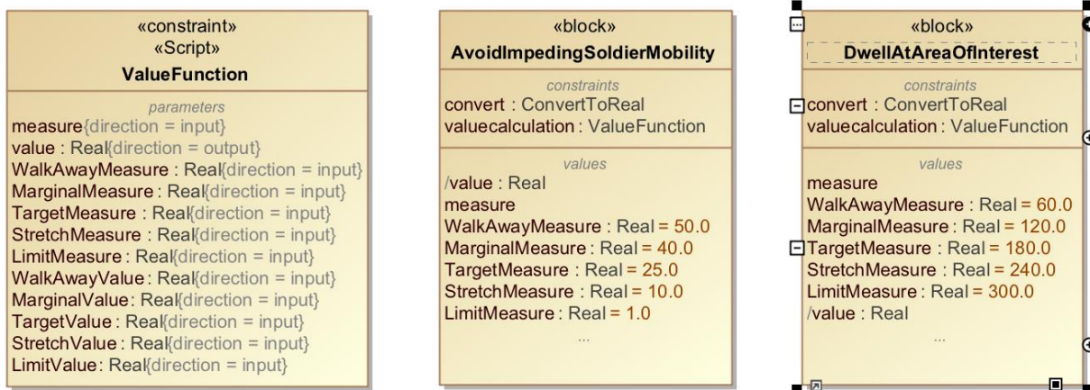
Figure 6. Constraint block defining the value function and two examples of value blocks associated with the UAS.
