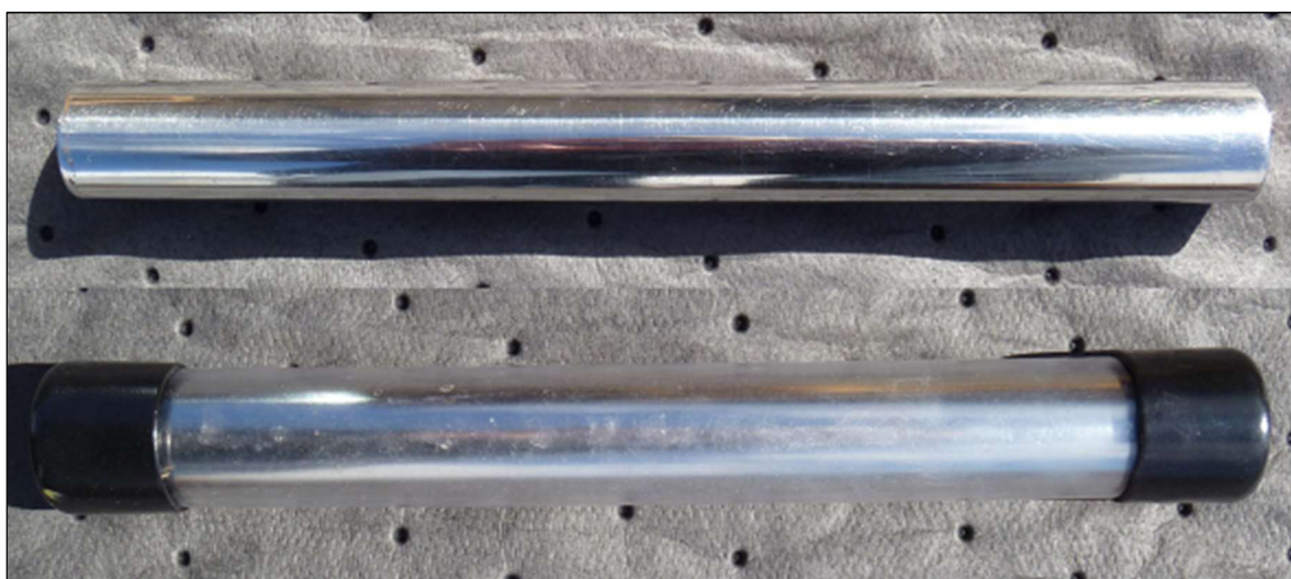
Figure 13. One of the high field (powerful) permanent REE magnets used in this study (top) and housed in the sheath with endcaps (bottom).
