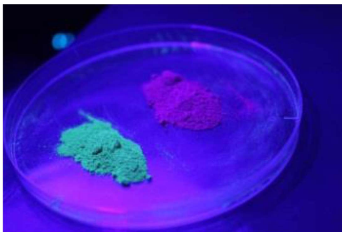
Figure 8. The green and pink tracers photographed under blue light illumination (395 nm). The green tracer appears to generate a 'stronger' fluorescent emission as the peak emission spectra is closer to the wavelength of the blue light in comparison to the pink tracer peak emission spectra.
