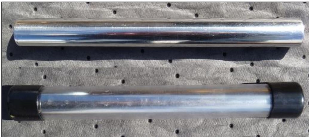
Figure 29. One of the magnets used in this study (top) and housed in the sheath with endcaps (bottom). For scale, the bar magnets are 30 cm in length.
