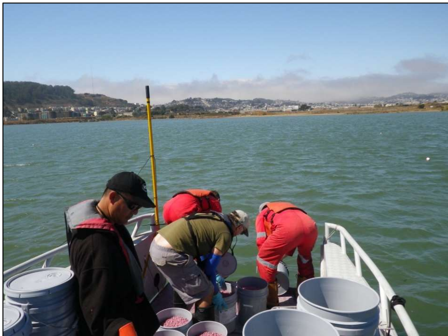
Figure 20. Partrac and SPAWAR staff deploying the tracer.
