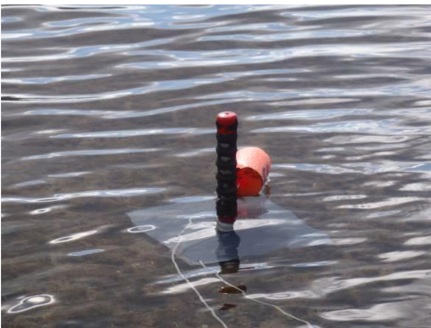
Figure 8. A vertical bed-frame mounted magnet to capture tracer moving in the bottom boundary layer at the second demonstration site.
