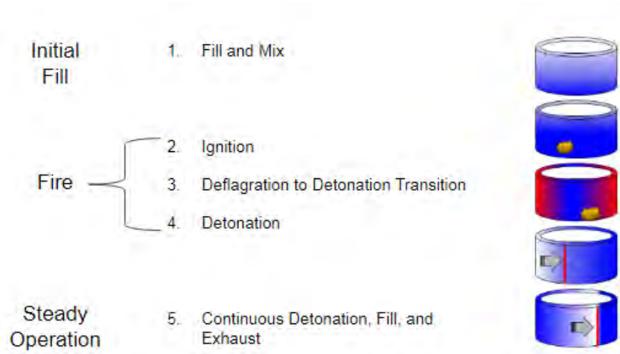
Figure 2. RDE Detonation Process [21]
