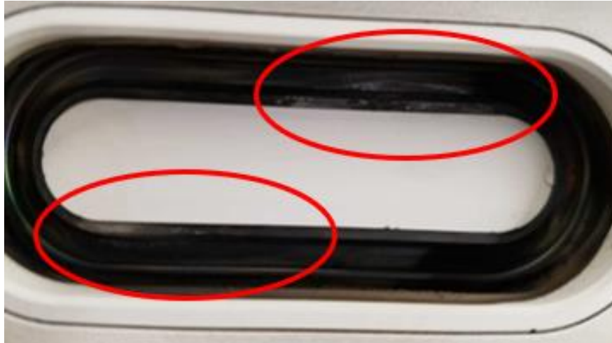
Figure 41: Visual Erosion on Channel
