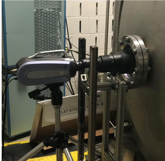
Figure 14: High speed camera set-up
