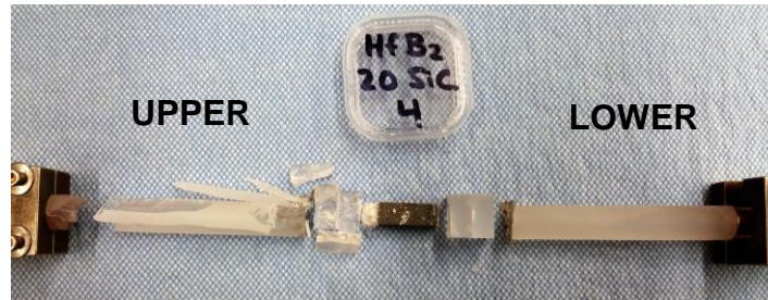
Figure 11. Failed YAG rods and sapphire spacers used in a creep test of specimen HfB 2 -20SiC-4 performed at 150 MPa for 8.05 hours.
