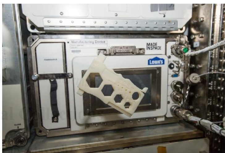
Figure 6: The Additive Manufacturing Facility printed the Future Engineers Multi-tool (in foreground) while installed in the International Space Station.
