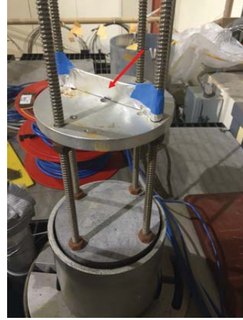
(b) Foil pack attached to rig for insertion into Co-60 source
