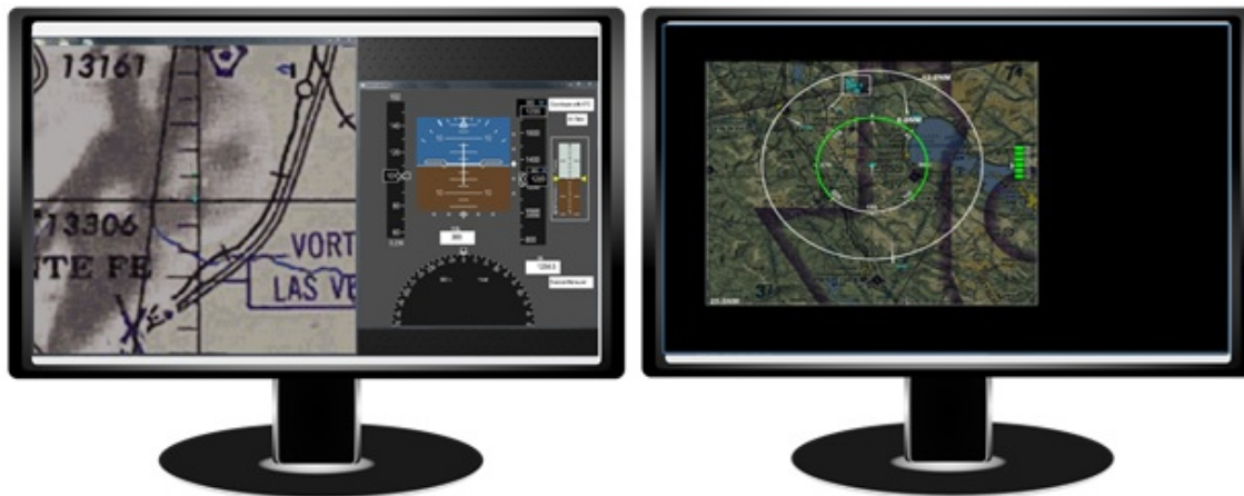
Figure 1. Experiment 1 pilot workstation displays. The multifunction display on the left includes a moving map and the PFD. The DAA display is on the right.
