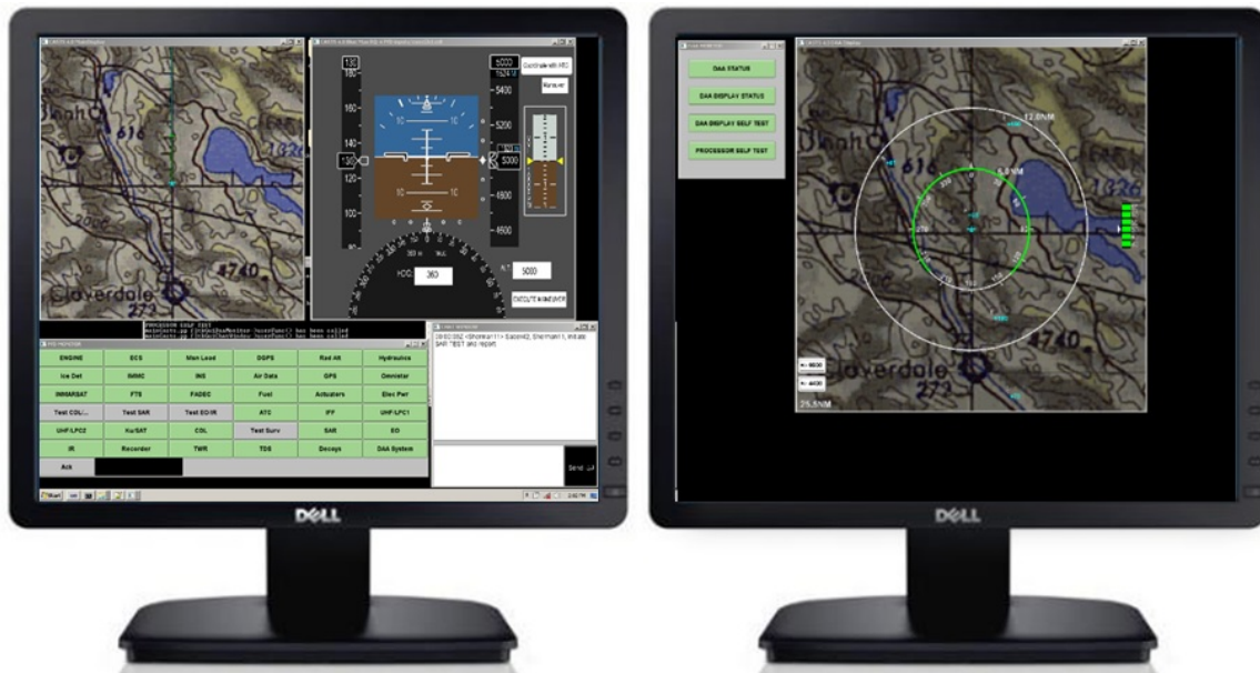
Figure 2. Experiment 2 pilot workstation displays. The multifunction display on the left includes a moving map, the PFD, system status indicators, and the chat window. The DAA display is on the right.
