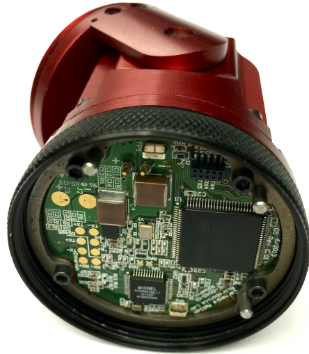
Figure B.4: Photo of the modular SEA Snake interface. Dowel pins provide alignment while the threaded collar mechanically secures and seals the modules. The electrical connection is made with spring-pin connectors touching target areas on the control board.
