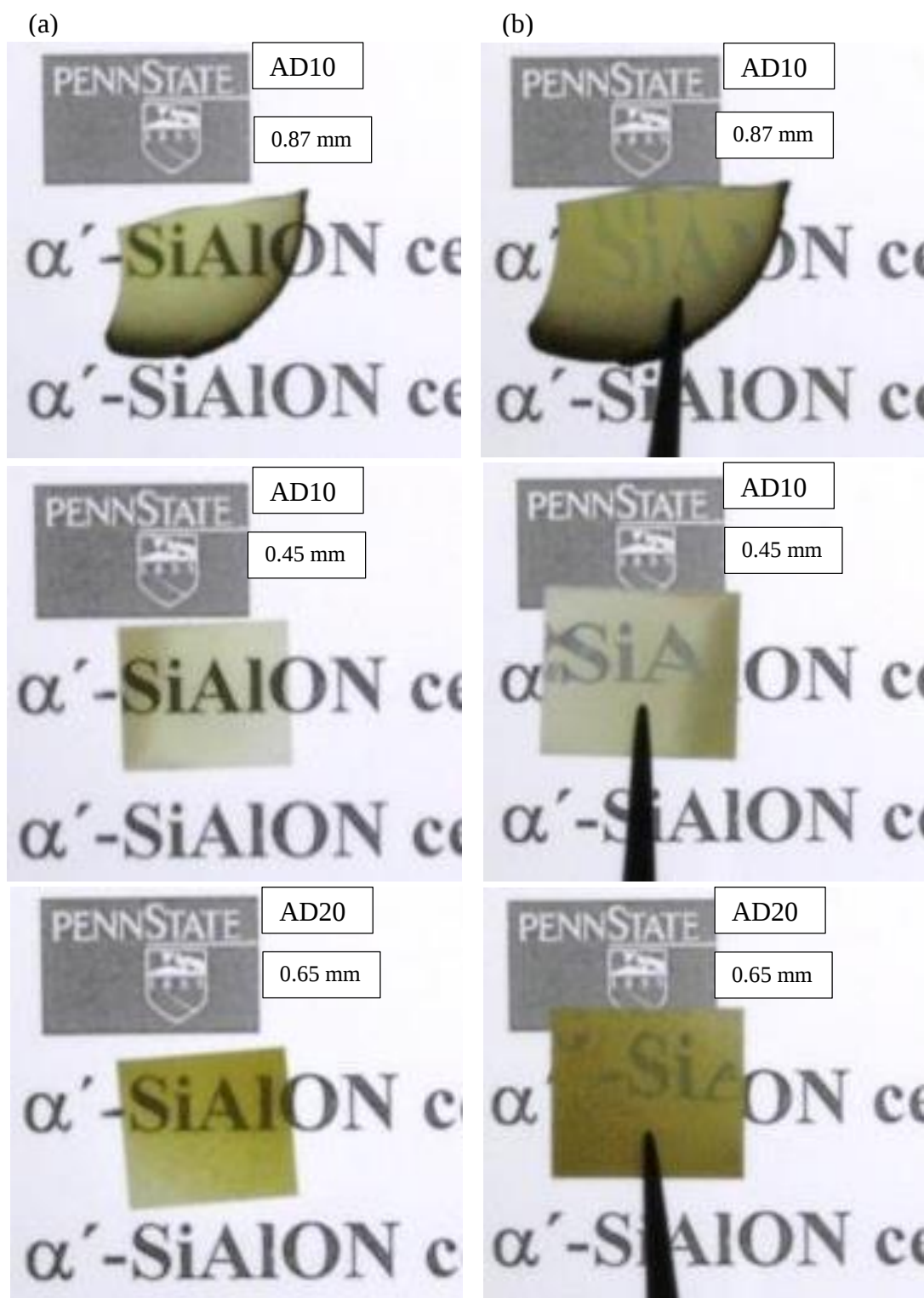
Figure 3.17 - The light transmission of the AD samples. Relatively higher in-line transmission is seen in samples with clearer text when placed above the backlit light. (a) The sample is placed directly on a backlit background. (b) The sample is 10 cm above the backlit background. The AD10 samples have a slight curvature which is causing the text to warp. The camera is 64 cm above the background text.
