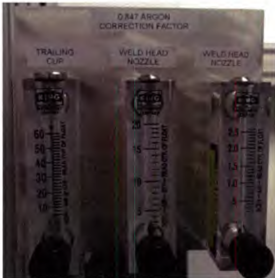
Figure 4.1.0-3. Auxiliary Control Panel (top), argon flow is regulated by flow rate (bottom left), and cooling air flow is pressure regulated.
