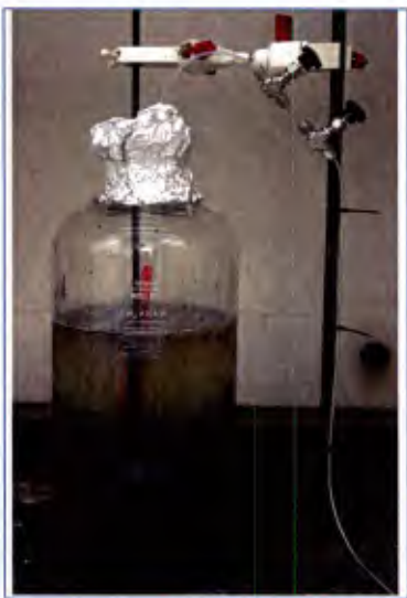
Figure 3.1.9 Pyrex bottle used to incubate samples. Sediment depth was 13.1 cm; 4 liters of water.
