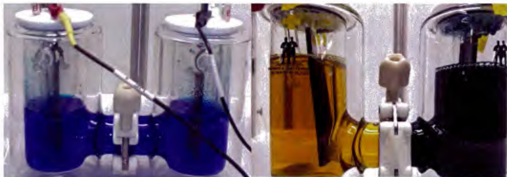
Figure 2.1.14. The electrolysis cell for vanadium (II), (III), and (V) electrolytes preparation.
