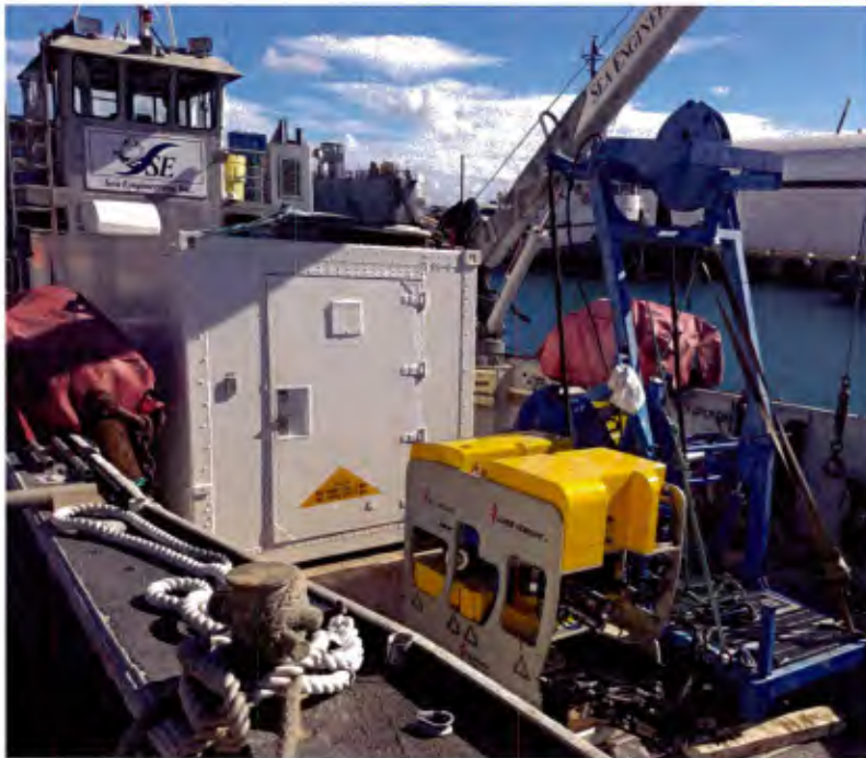
Figure 4.2.4. Super Mohawk ROV and control van aboard Sea Engineering, Inc. vessel Huki Pau in Honolulu Harbor, during initial sea trials.
