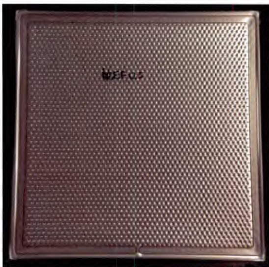
Figure 4.1.12. A TFHX weld certification sample. Weld certification samples were used to demonstrate the success of foil-foil welds and establish patterns that would meet the required pressure rating.
