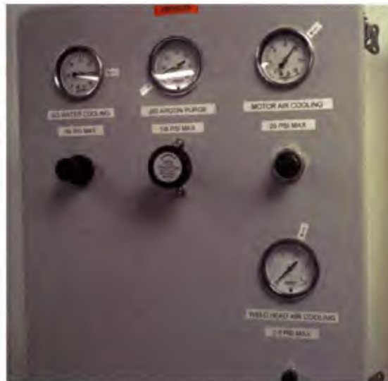
Figure 4.1.0-3. Auxiliary Control Panel (top), argon flow is regulated by flow rate (bottom left), and cooling air flow is pressure regulated.
