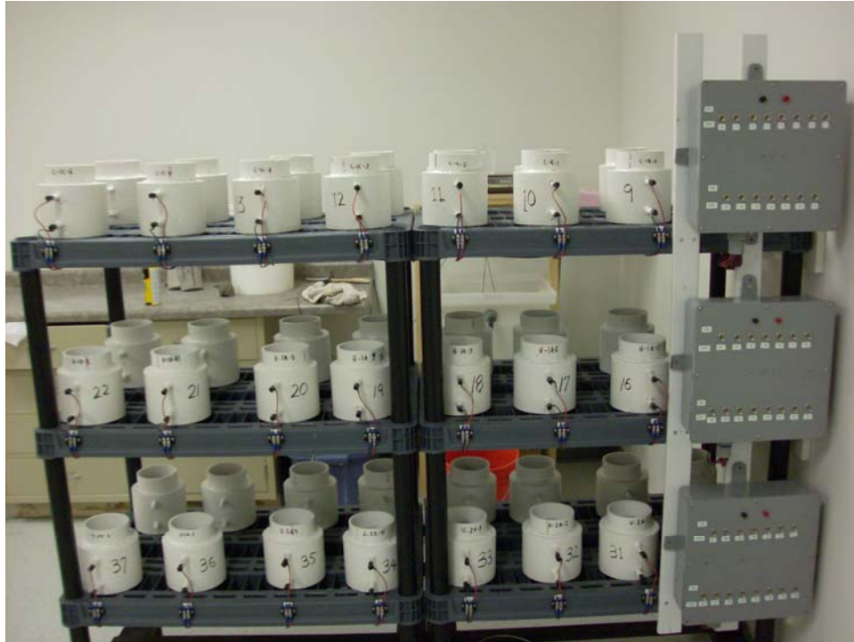
Figure 1 – Photograph of chloride threshold experimental setup
