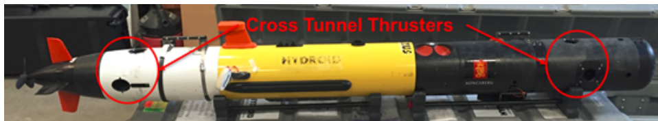
Figure 1.2. Location of CTTs on a REMUS Vehicle. Source: [1].
