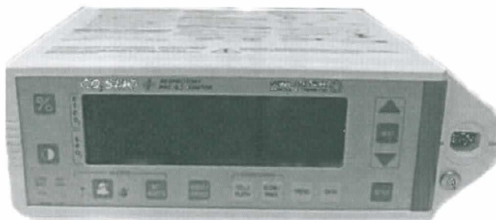
Figure 2.2: This is the respiratory profile monitor used in the system. It uses a CO 2 /flow sensor to read several different parameters including resistance and compliance. It is connected to the computer via a serial port.
