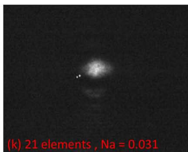
Figure 45: Far field images of SBN:61 waveguides at 1550 nm.
