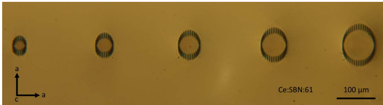
Figure 42: Transmission microscope image of depressed cladding waveguides in Ce:SBN:61. The inscription laser was parallel to the a-axis of the crystal. Inscription parameters were 100 kHz, 1.1 ps, 0.3 \mu J for top half, 0.35 \mu J for bottom half, number of elements are equal to diameter in \mu m multiplied by 3/5 and 0.68 NA lens. The waveguides had a diameter of 30, 40, 50, 60 & 75 \mu m respectively from left to right of the figure.
