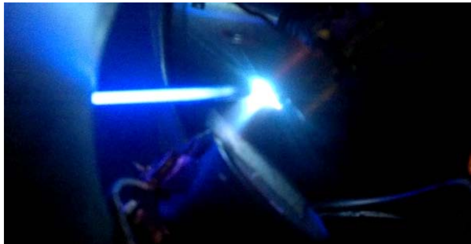
Figure 4.3 PPD system in operation with visible plume of ablated material.
