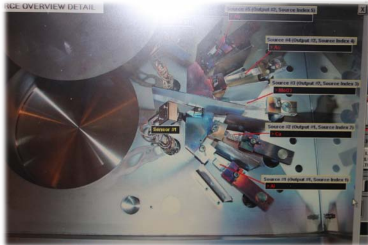
5 Source Metals Evaporator with E-Beam Upgrade Capability
