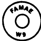
A112 CHILE On 9x17-mm pistol cartridges. The W stands for Walther. See Note 4.
