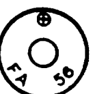
A111 UNITED STATES Frankford Arsenal. Typical marking on 7.62x51-mm NATO cartridges. See Note 4.
