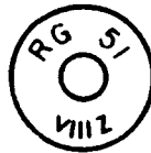
A347 UNITED KINGDOM Made at R.O.F. plant at Radway Green. 1951. See Note 3.
