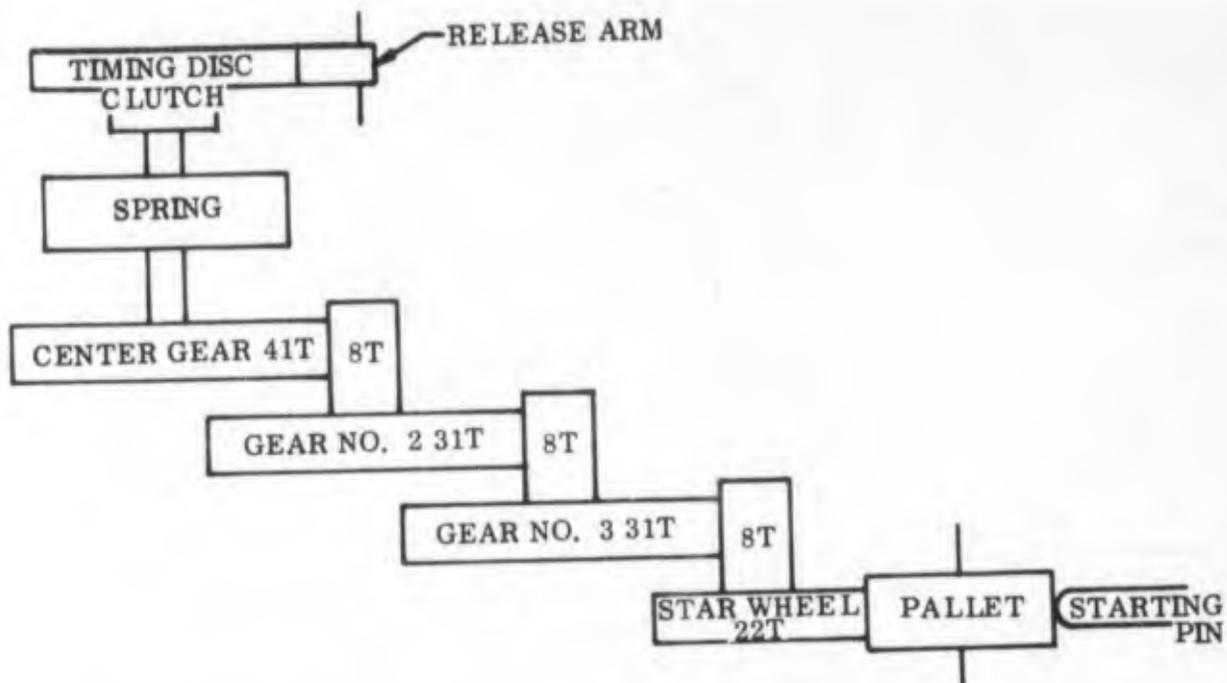
Figure 15. FMU-54A/B Fuze Timer Gear Schematic Diagram
