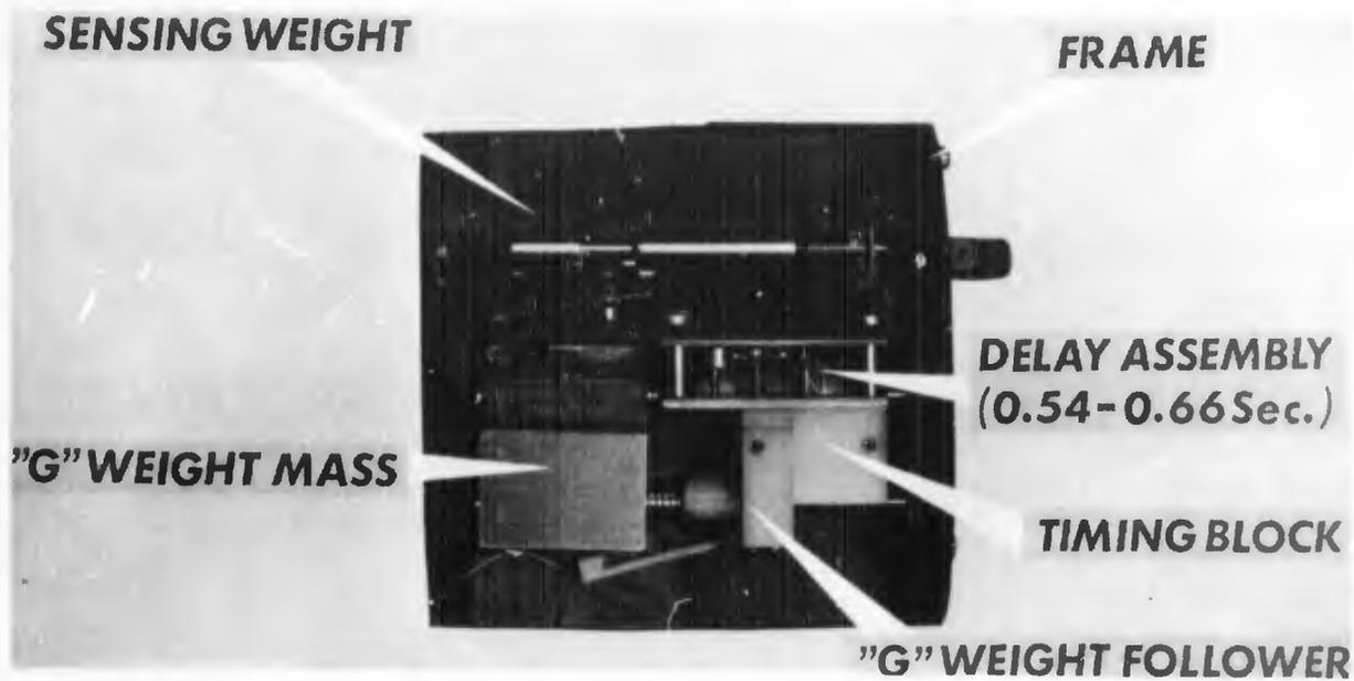
Figure 25. FMU-70/B Fuze Retard Sensor Breakaway Functioned
