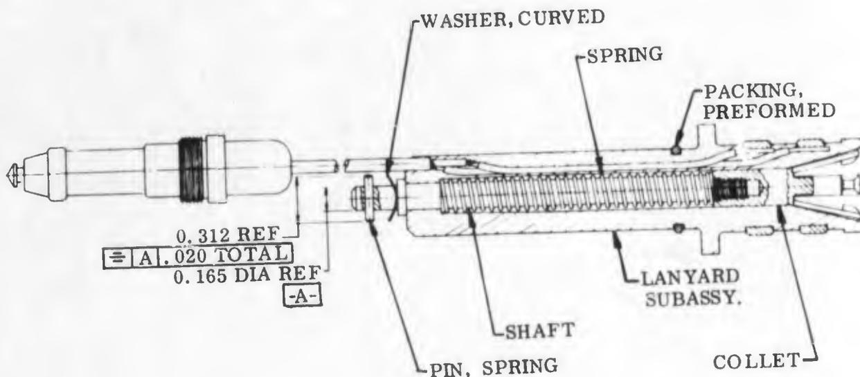
Figure 9. Lanyard Assembly
