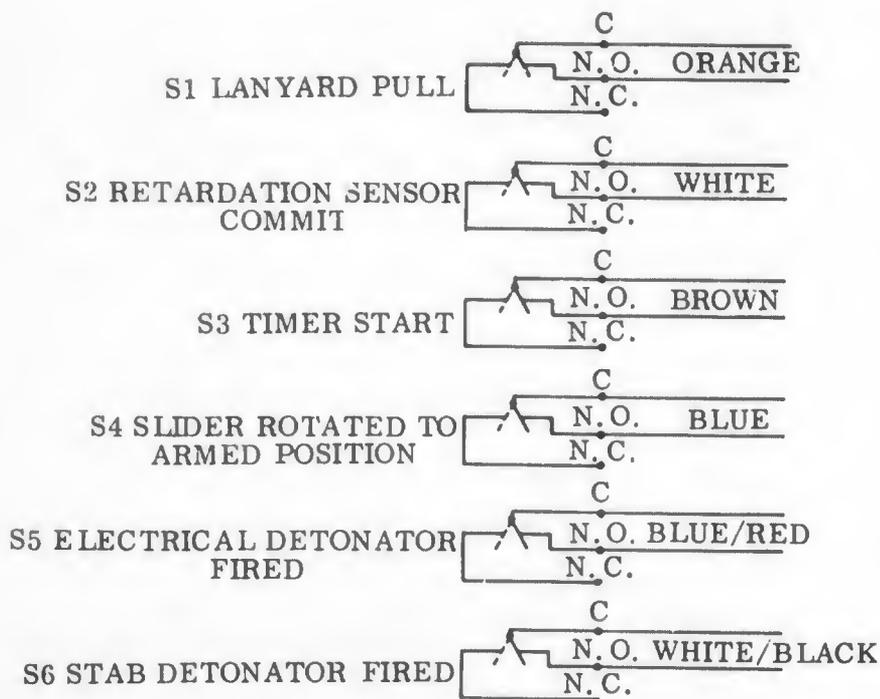
Figure 20. Telemetering Switch Schematic Diagram
