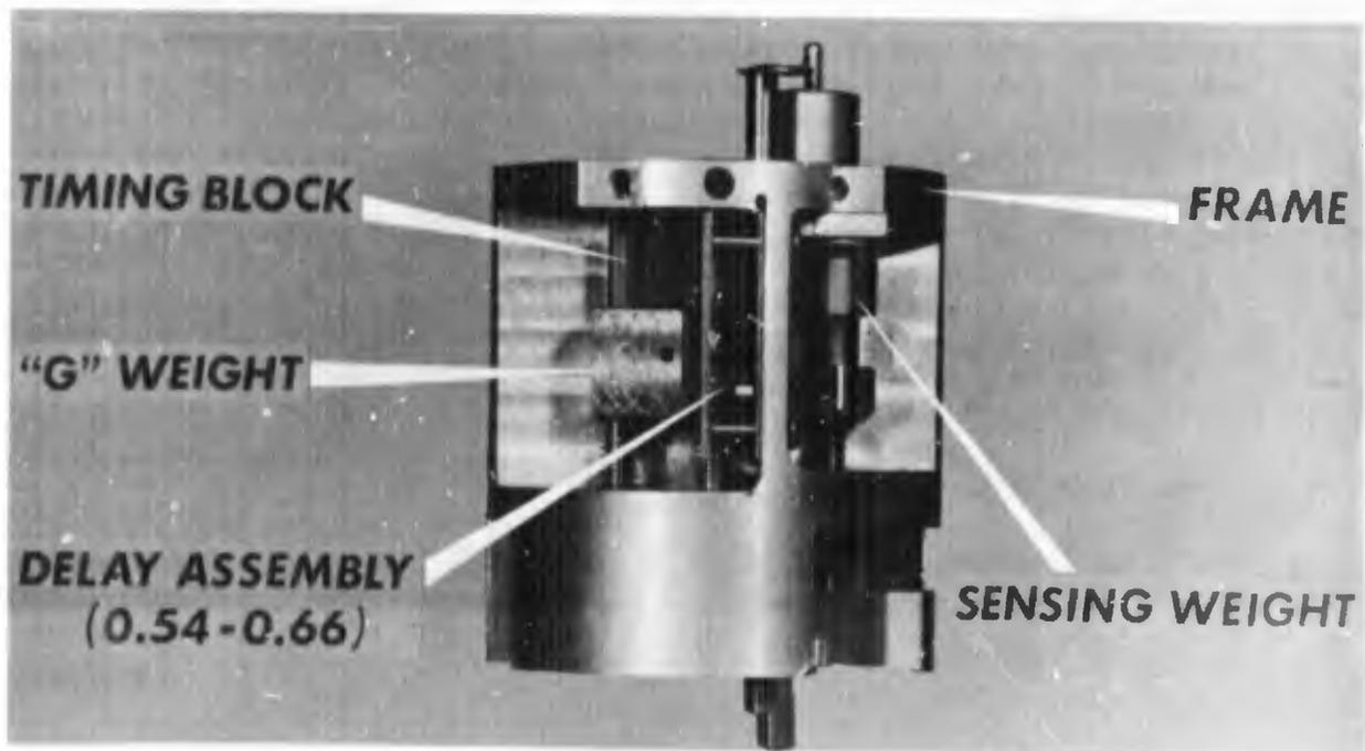
Figure 11. FMU-54A/B Fuze Frame Assembly Showing Retard System
