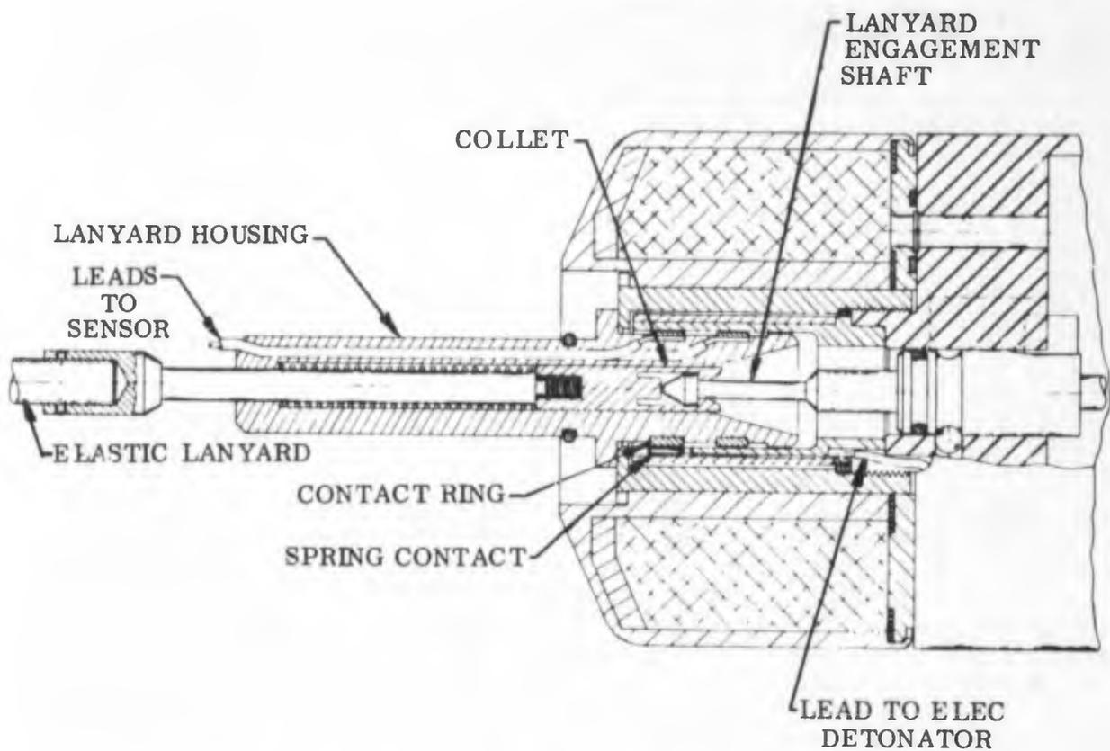
Figure 10. FMU-54A/B Fuze Housing and Lanyard Assembly
