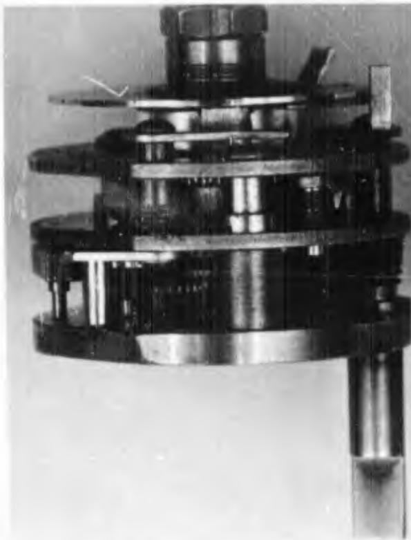
Figure 14. FMU-54A/B Fuze Timer Assembly - Side View
