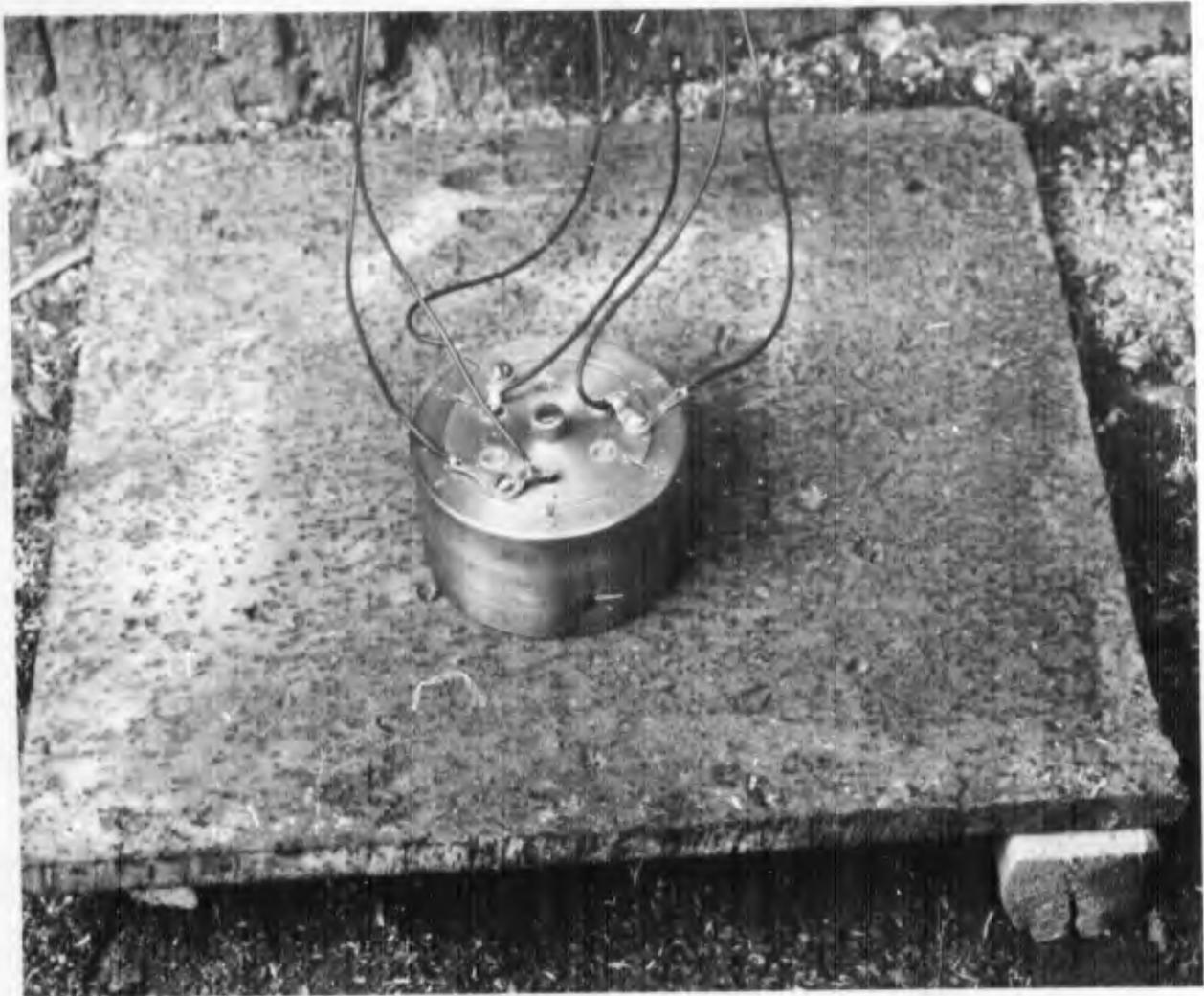
Figure 29. Explosive Test Set-up (Electrical Detonation)
