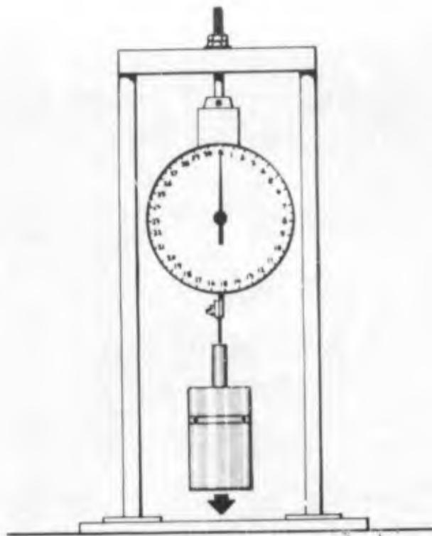
Figure 26. Lanyard Pull Test Set-up
