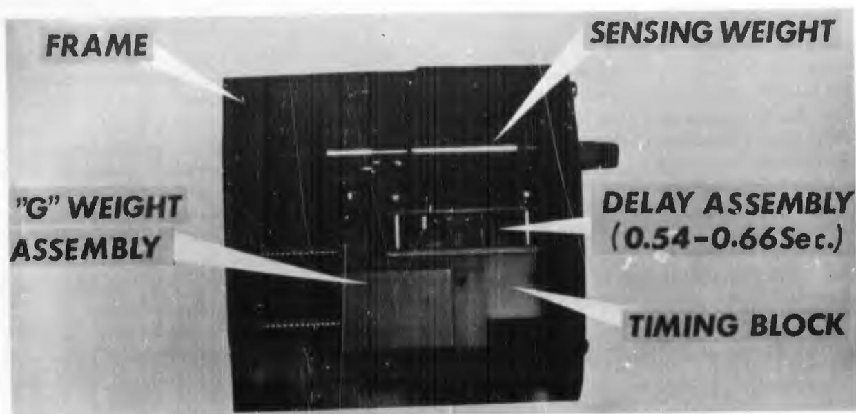
Figure 23. FMU-70/B Fuze Retard Sensor Locked - No Retard
