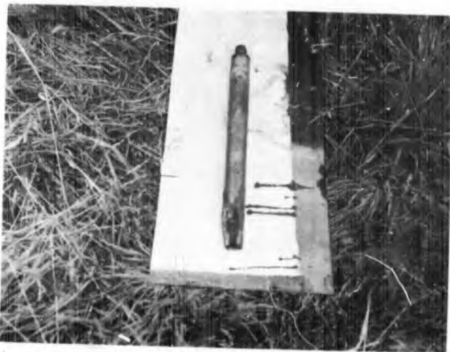
Figure 51. Shelby tube with "spun" edge damaged by driving.
