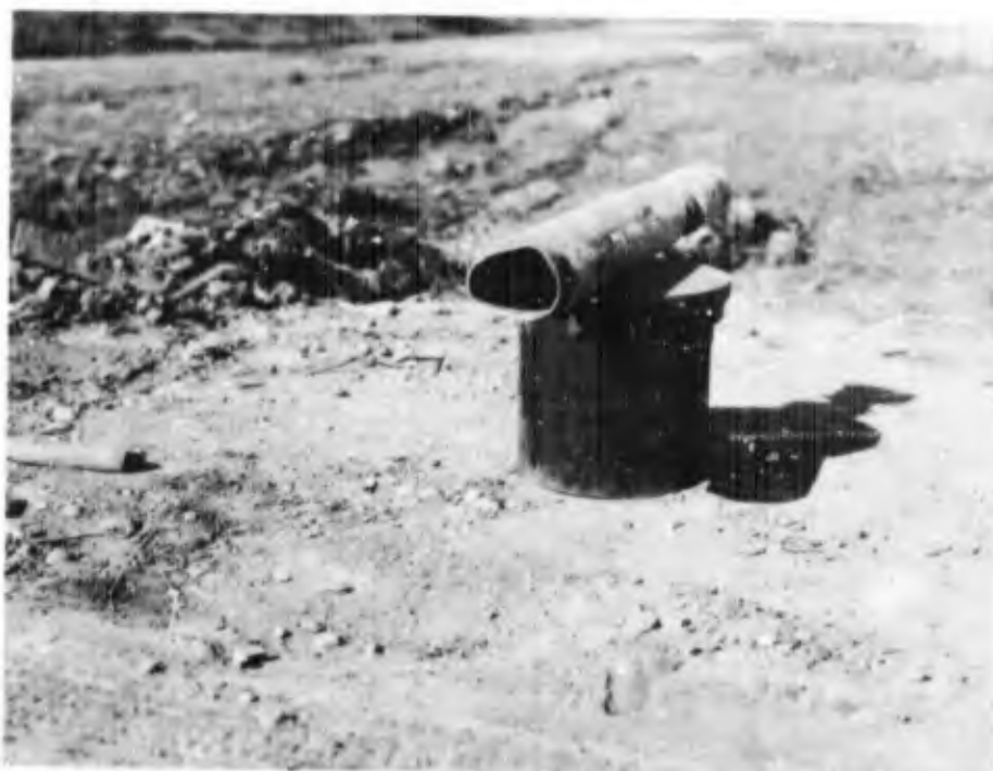
Figure 35. Acker solid tube sampler after failure.
