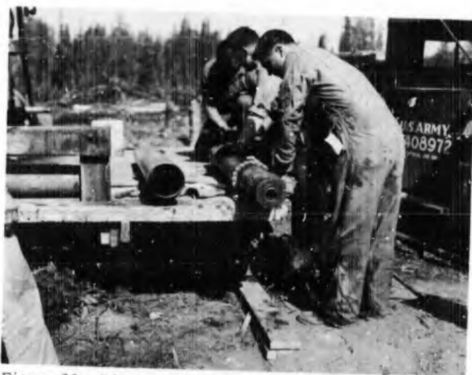
Figure 23. Disassembling core barrel to remove sample.
