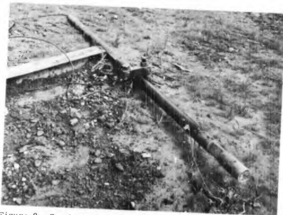
Figure 8. Sectional sinking bar (4 in. x 10 ft) complete with casing driving clamps.
