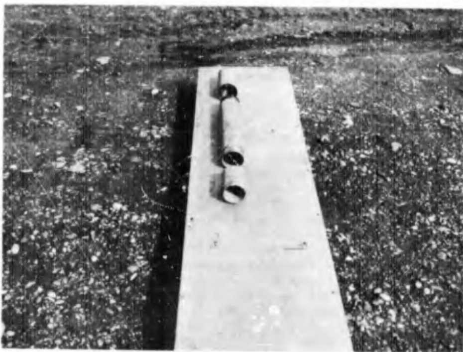
Figure 44. Disassembled Sprague and Henwood solid tube sampler.
