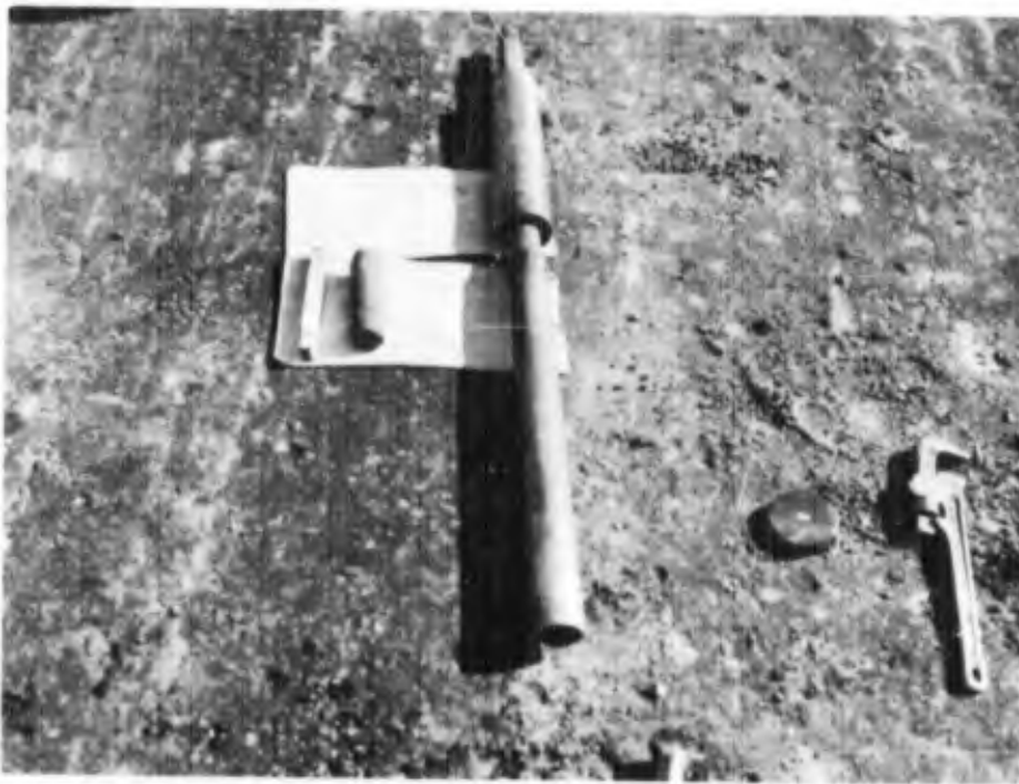
Figure 53. Drive arrangement for shallow soil sampling.
