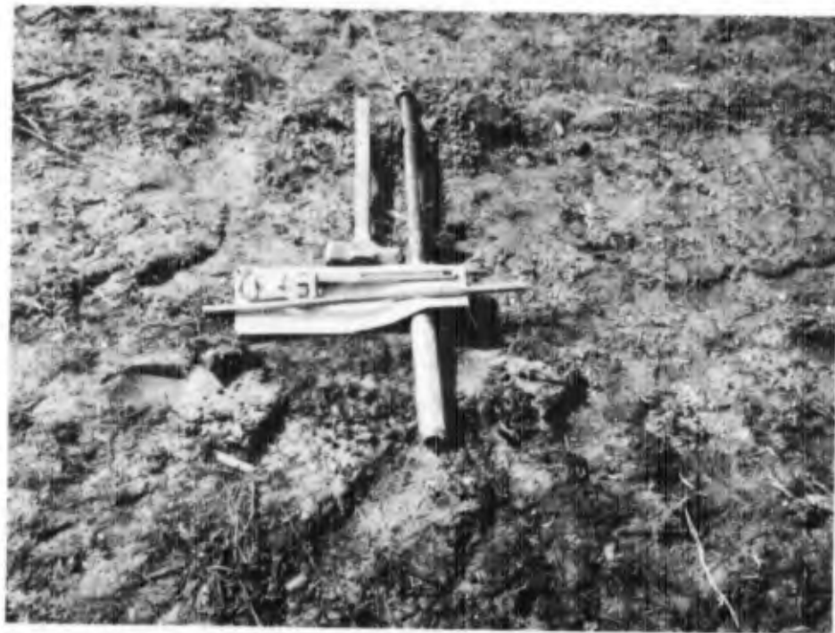
Figure 36. Acker split tube sampler, 1\frac{1}{2} in. ID and 2 in. OD, and driving equipment.
