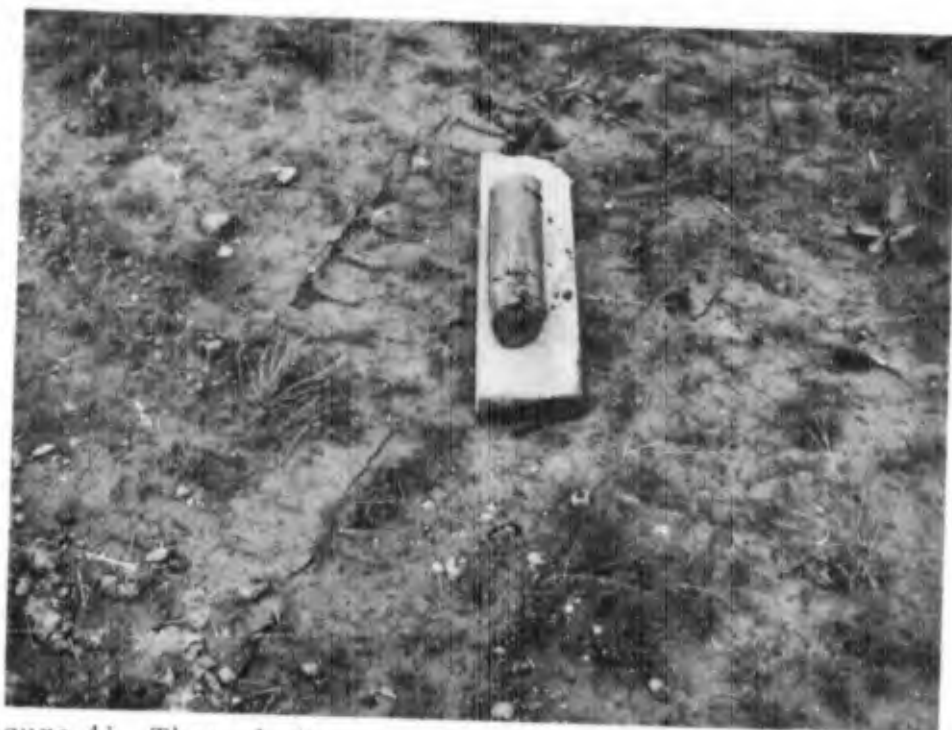
Figure 41. Thawed silt core recovered with steel pipe sampler.
