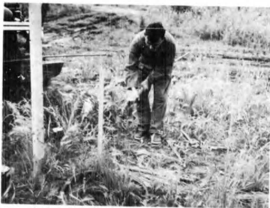
Figure 48. Driving thin walled electrical conduit sampler.
