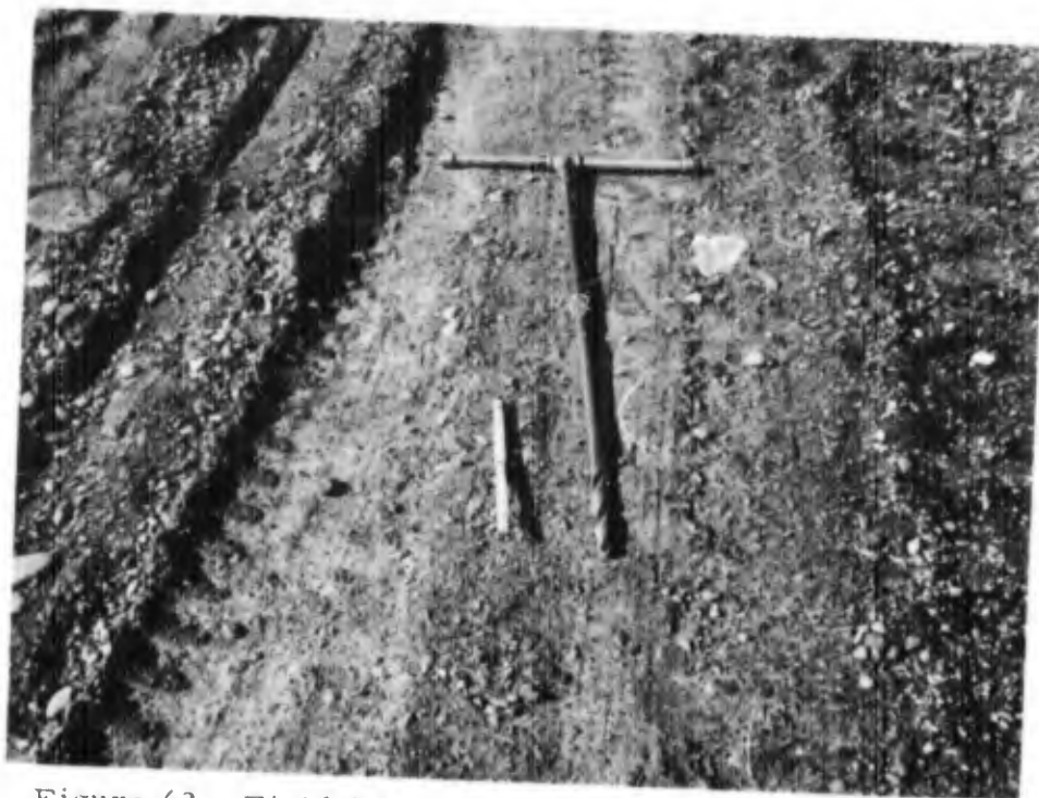
Figure 62. Field fabricated probing auger using 7/8-in. machine or twist drill.
