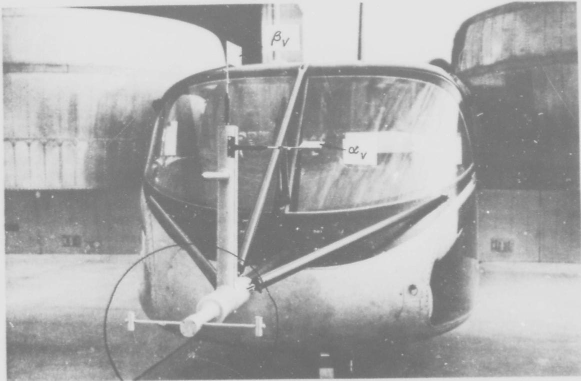
Figure I-15 VERTICAL VELOCITY LORAS INSTALLATION ON NOSE BOOM
