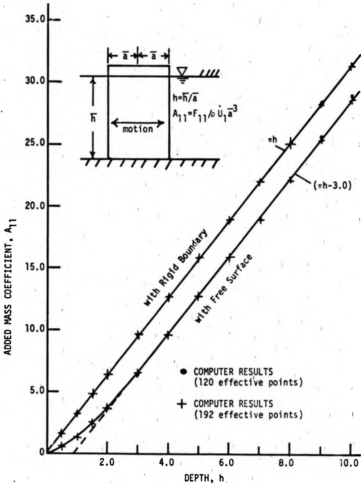
Fig. 8 - Added mass coefficient for a vertical circular cylinder.
