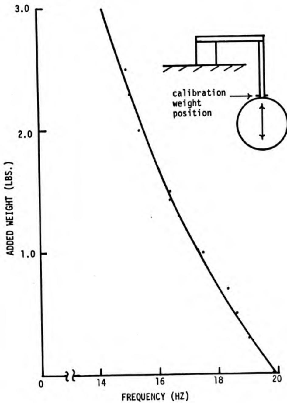
Fig. 13 - Calibration curve
