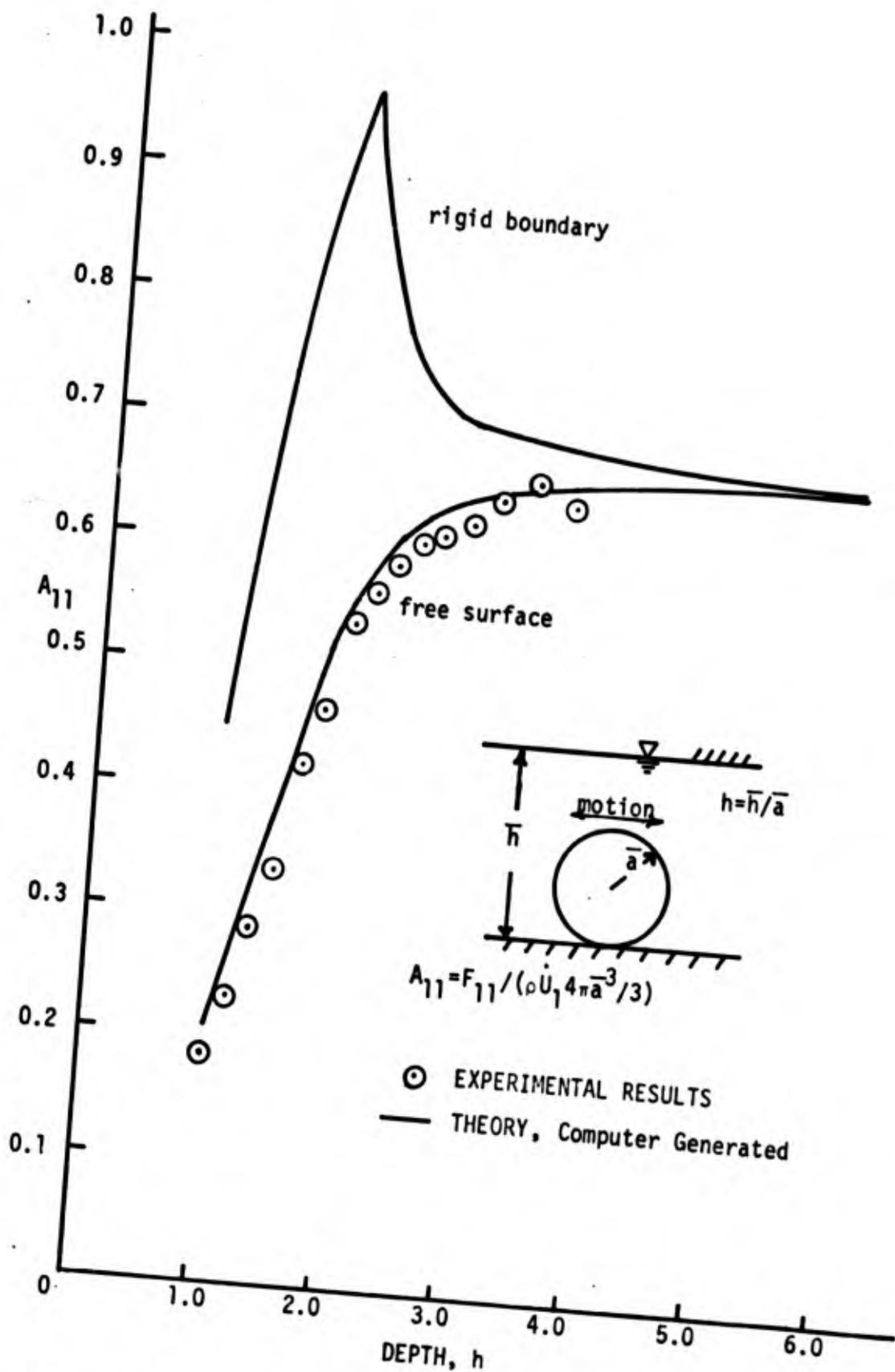
Fig. 17 - Added mass coefficients for a ball-mounted sphere.
