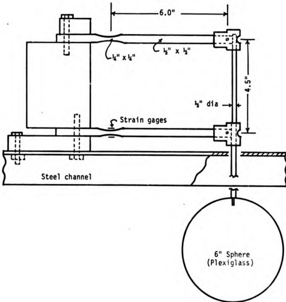
Fig. 5 - Experimental apparatus used in heave tests.
