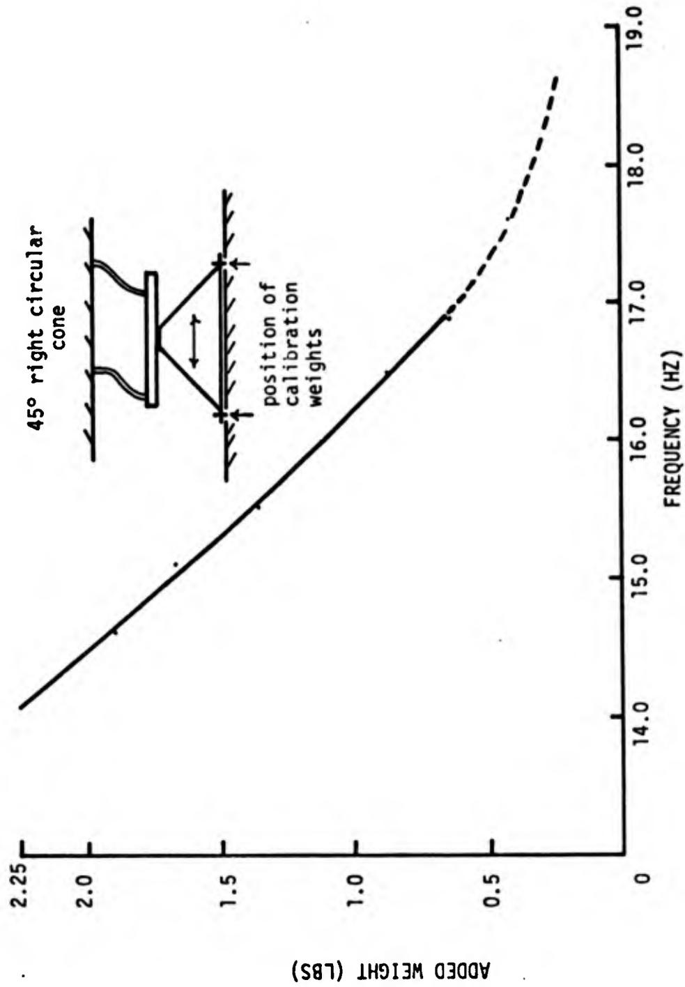
Fig. 20 - Calibration curve (Cone - Horizontal Motion)
