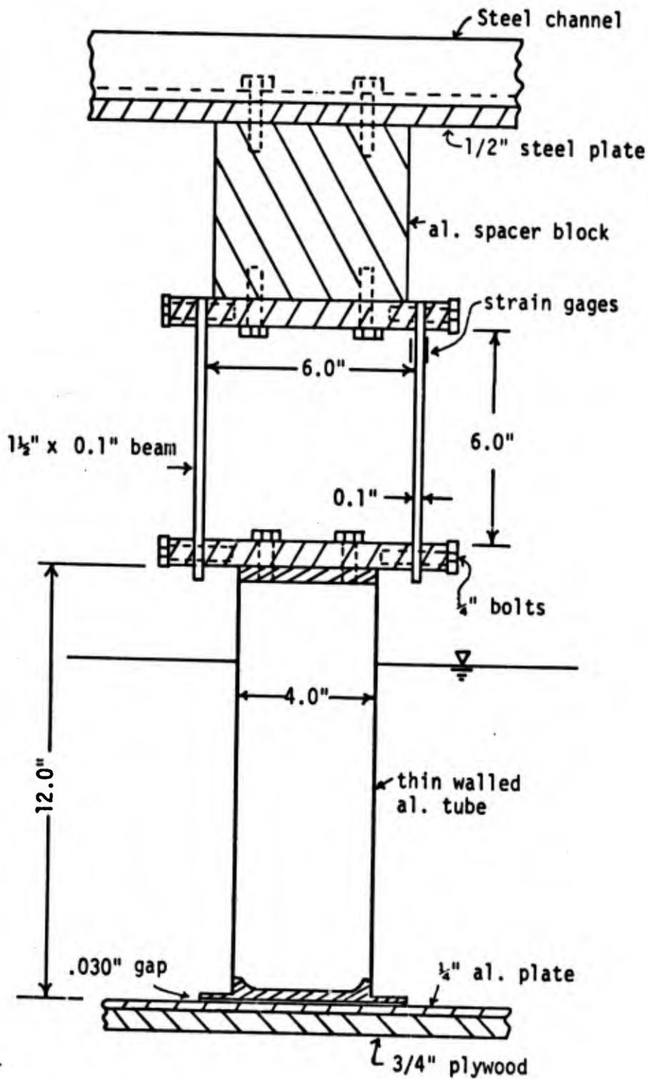
Fig. 3 - Experimental equipment.
