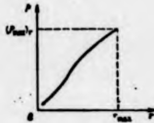
Figure 1.11. Determination of Optimal Limiting Control: V = \text{const}, H = \text{const}, d = \text{const}, r_{\text{opt}} = r_{\text{max}}
