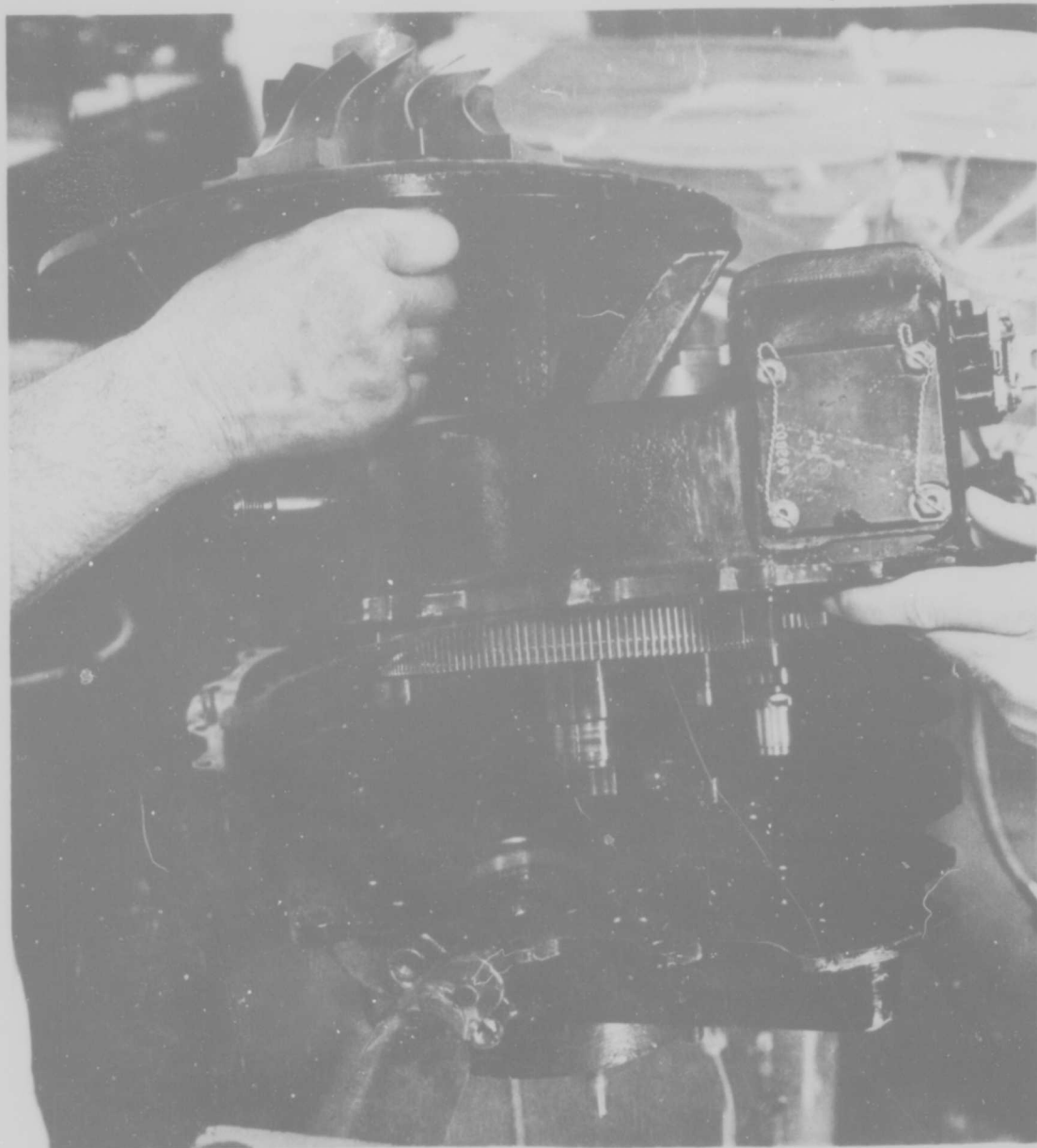
REMOVAL OF POWER SECTION FROM GEAR CASE LOWER HALF FIGURE 87
