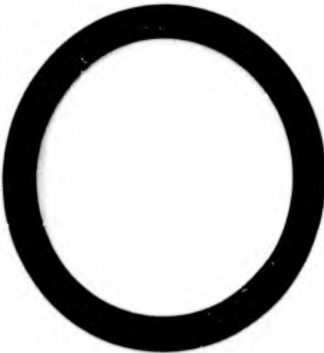
REPRESENTATIVE O-RING TEST SPECIMENS AFTER EXPOSURE TO SHELLDYNE-H FUEL FOR 70 HOURS AT 250°F
