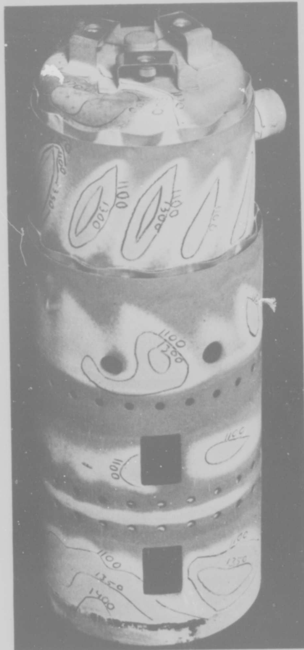
SHELLDYNE-H COMBUSTOR ISOTHERMS
