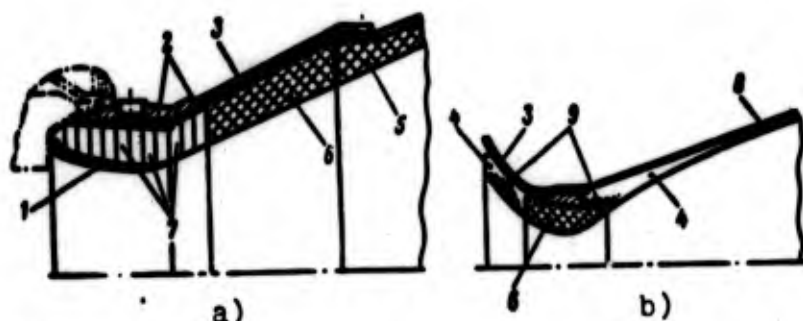
Fig. 18.11. Combined thermal insulation of nozzles: 1 - tungsten coating; 2 - insert made of pyrographite; 3 - steel shell; 4 - thermal insulation coatings; 5, 6 - graphite inserts; 7 - ring made of pyrographite; 8 - glass laminate shell; 9 - direction of layers of coating.
