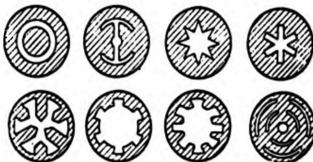
Fig. 5.14. Certain grain shapes with internal burning.
