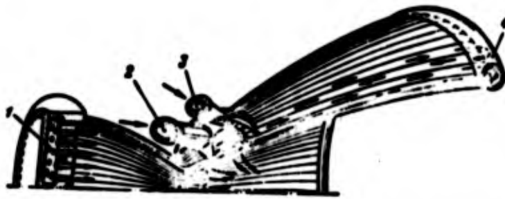
Fig. 12.22. Chamber of liquid propellant rocket engine with admission of gases from turbopump assembly into the nozzle: 1 - head of chamber; 2 - feeding of gases from turbine of the turbopump assembly; 3 - feeding of combustible (liquid hydrogen); 4 - annular collector for joining one inlet and two return tubes.
