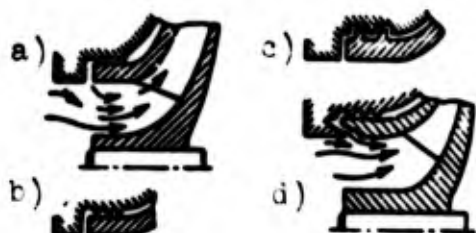
Fig. 14.11. Types of sealing for impellers: a) slot; b) labyrinth with lugs; c) labyrinth with rectangular teeth; d) labyrinth with a baffle.
