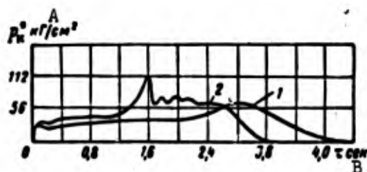
Fig. 6.5. Diagram of combustion process. 1) Stable process; 2) unstable process. A) \text{kgf/cm}^2 ; B) s.
