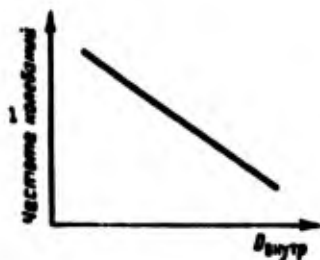
Fig. 6.6. Oscillation frequency as a function of inside diameter of hollow cylindrical grain. 1) Oscillation frequency.
