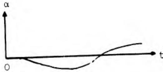
Figure 2.16. Change in angle of attack along active section of trajectory.
