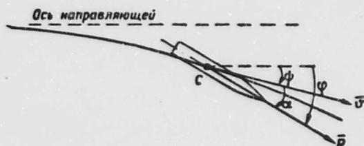
Figure 8.5. The angle determining oscillation of a rocket.
