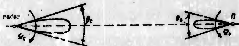
Fig. 10.30. Scanning method for determination of bearing.
