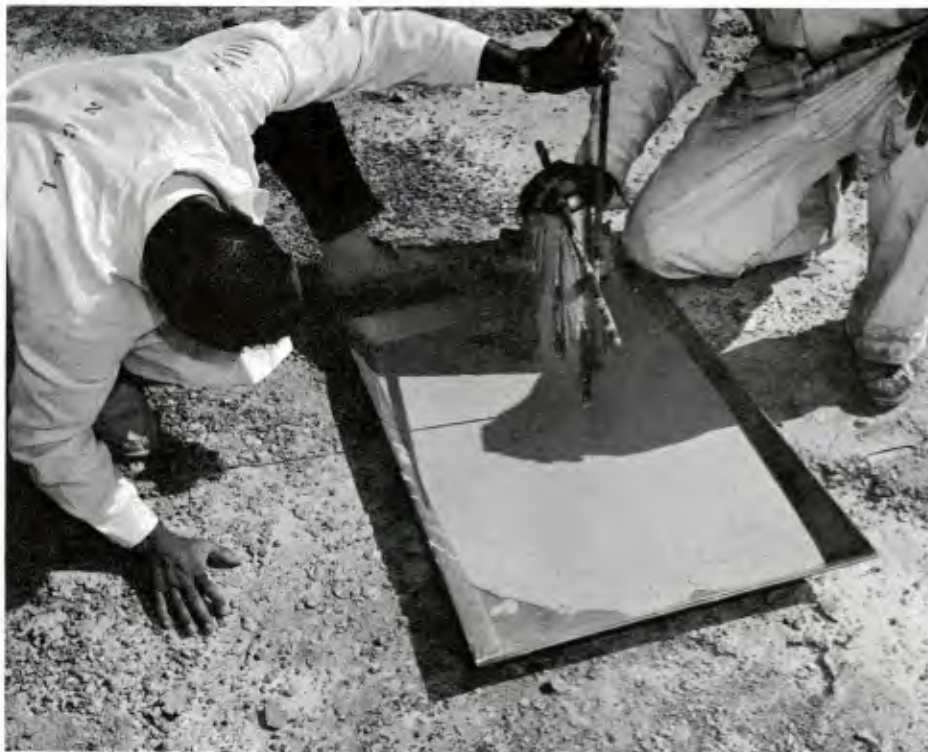
Figure 4. Typical slump test.
