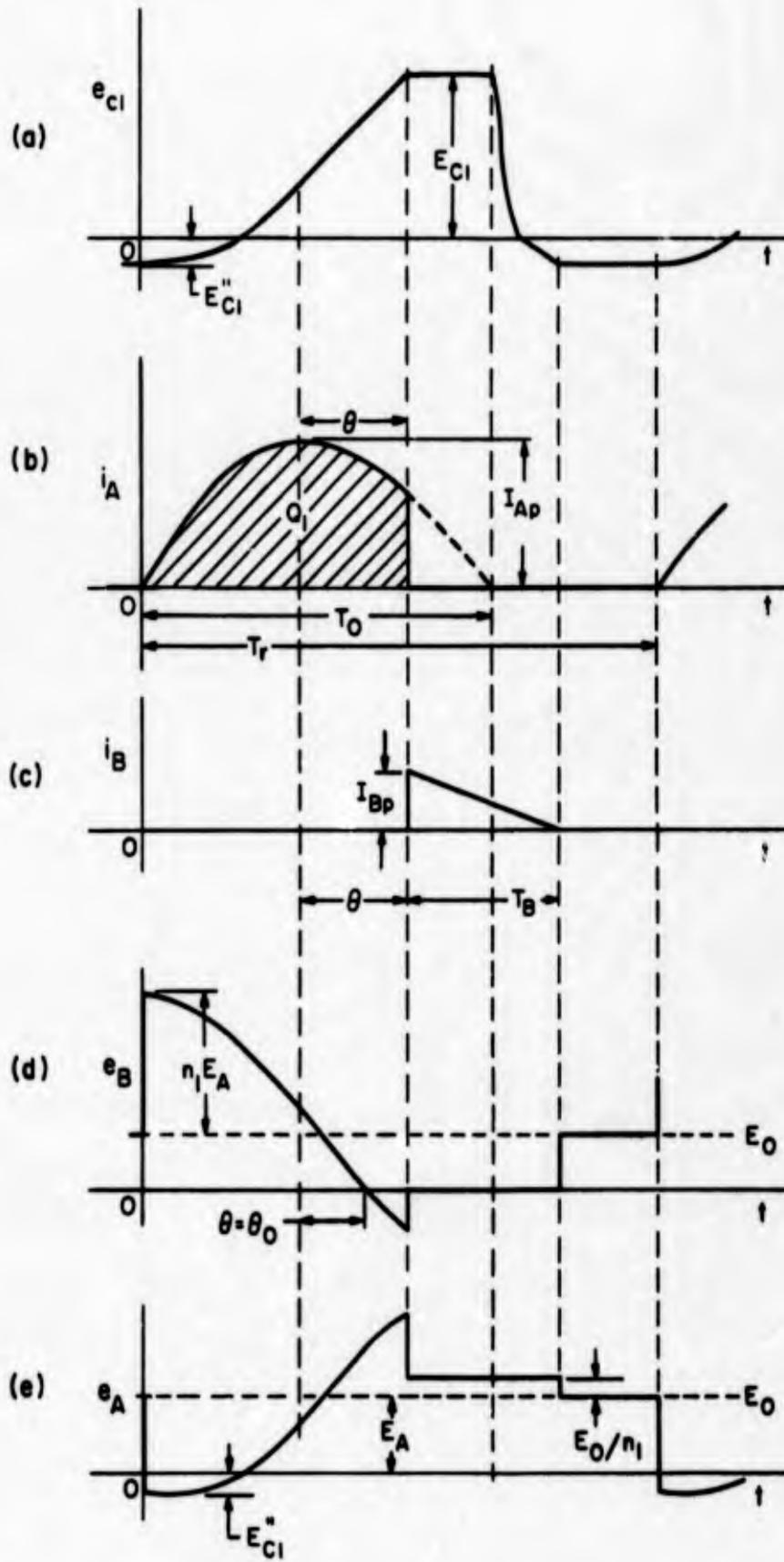
Fig. 3.7 Voltage-Regulator Waveforms
