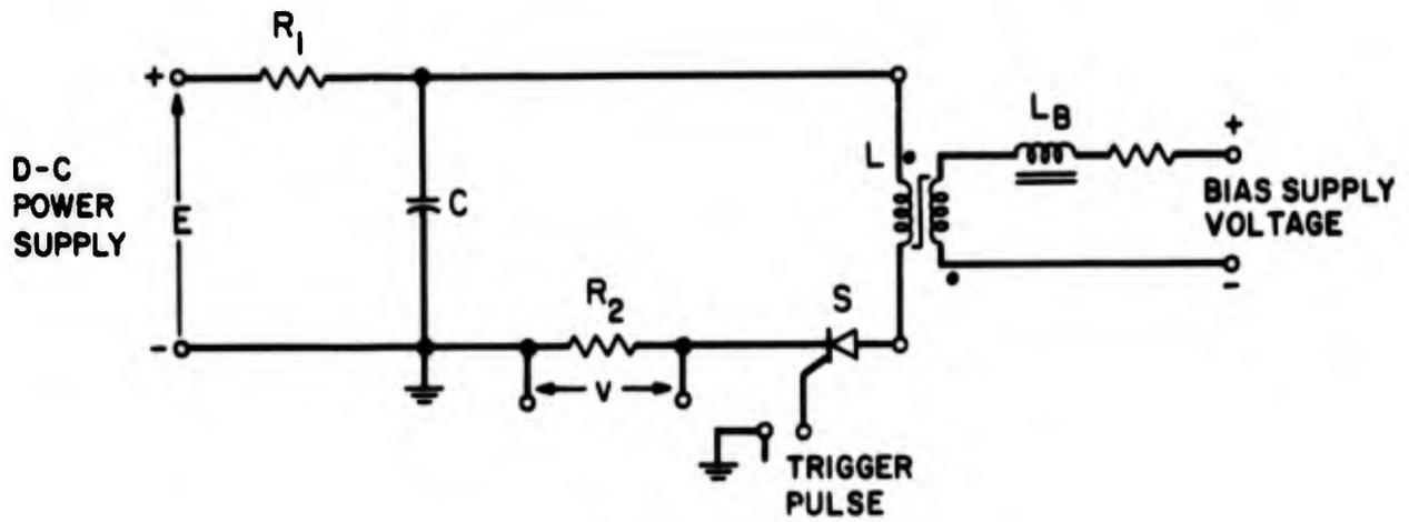
Fig. B.1 Saturable-Inductor Test Circuit
