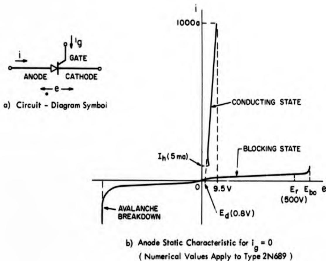
Fig. 2.3 Static Characteristic of Controlled Rectifier
