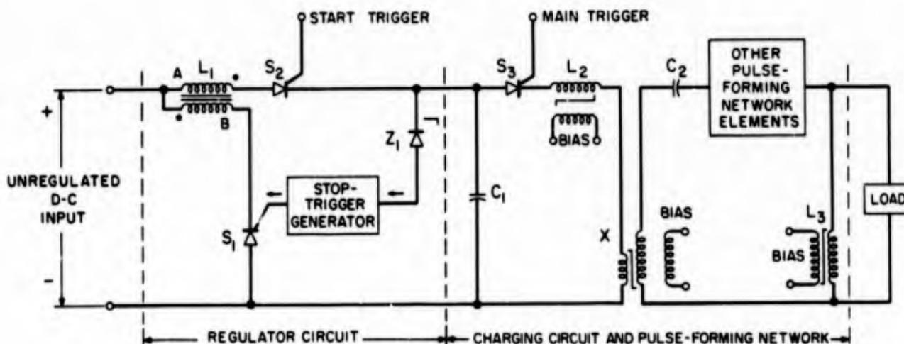
Fig. 1.3 Basic Circuit of the Semiconductor-Magnetic Pulse Generator
