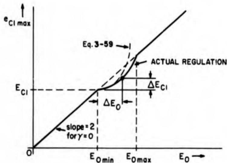
Fig. 3.9 Regulation Characteristic Showing Effect of  $L_{l1}$
