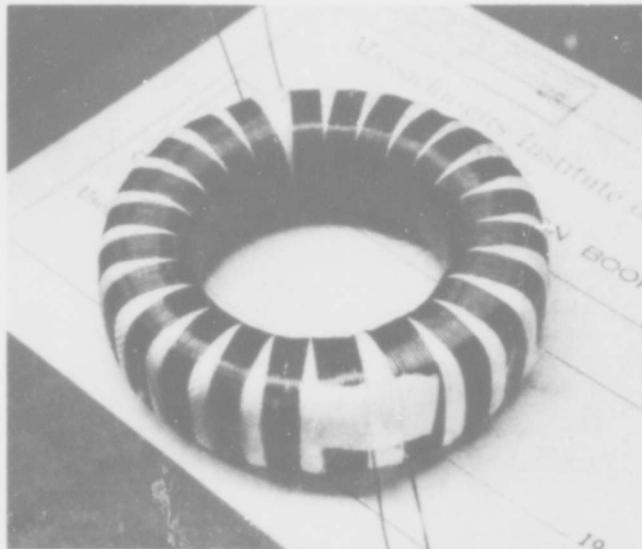
Fig. 5.12 Diode Inductor  $L_3$  High-Voltage Winding Construction
