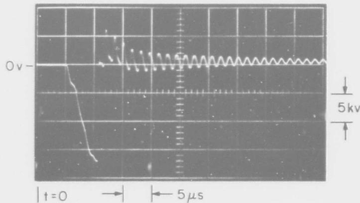
Fig. 5.4 Voltage  $e_X$  (Across Transformer High-Voltage Winding)
