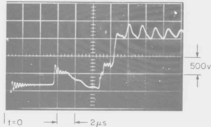
Fig. 5.10 Bias inductor  $L_b$  Voltage  $e_b$
