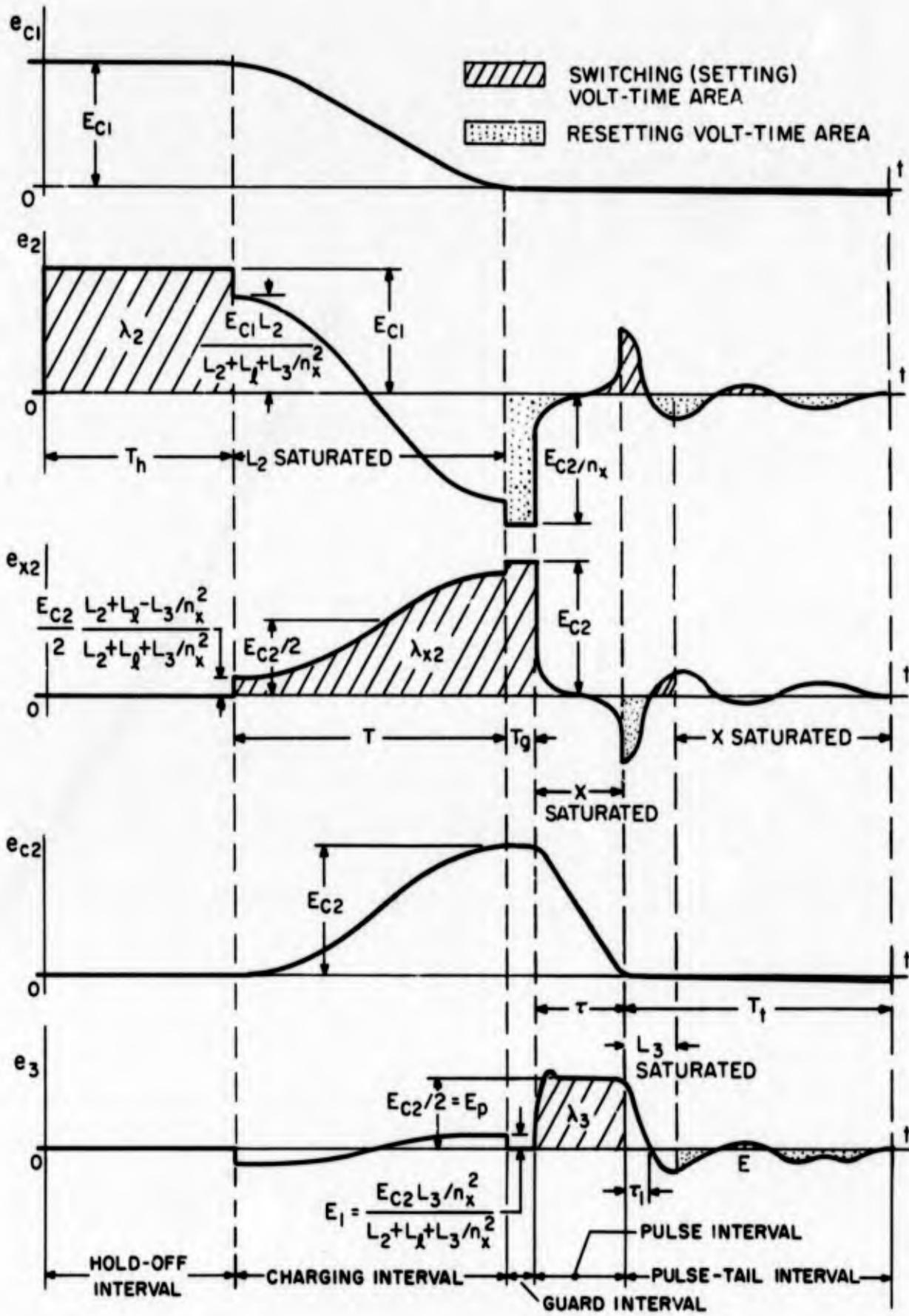
Fig. 3.5 Charging-Circuit Waveforms--R-F-Tube
