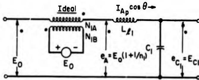
Fig. 3.8 Equivalent Circuit Showing Effect of  $L_{l1}$
