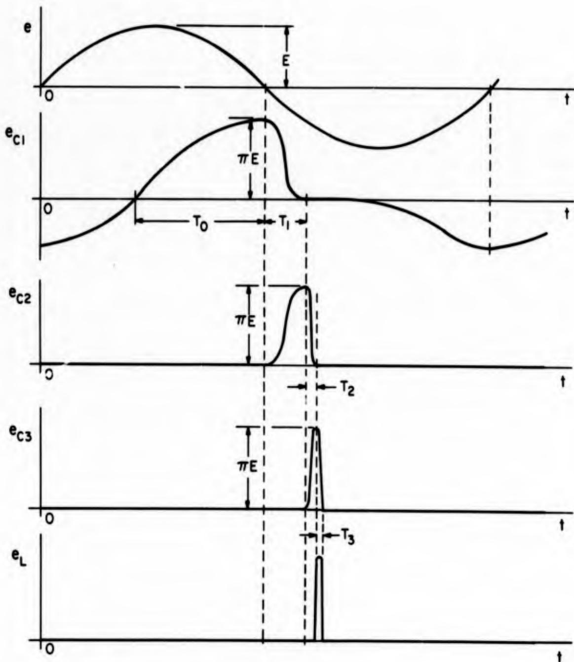
Fig. 1.2 Waveforms for Circuit of Fig. 1.1
