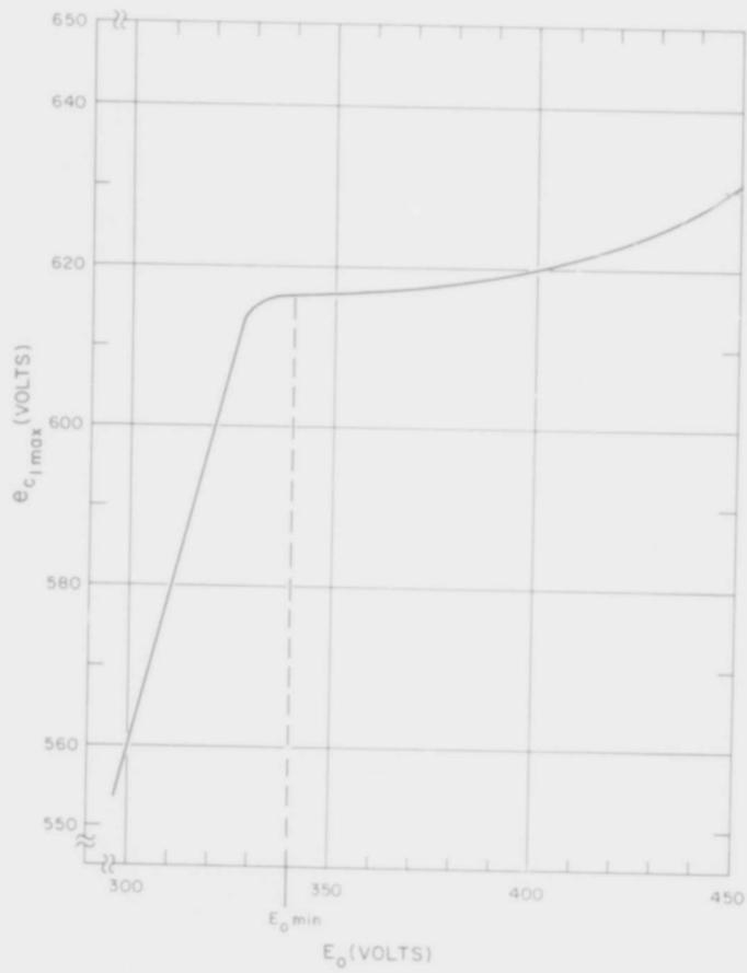
Fig. 5.8 Measured Regulation for  $E_{C1} = 612.5$  V
