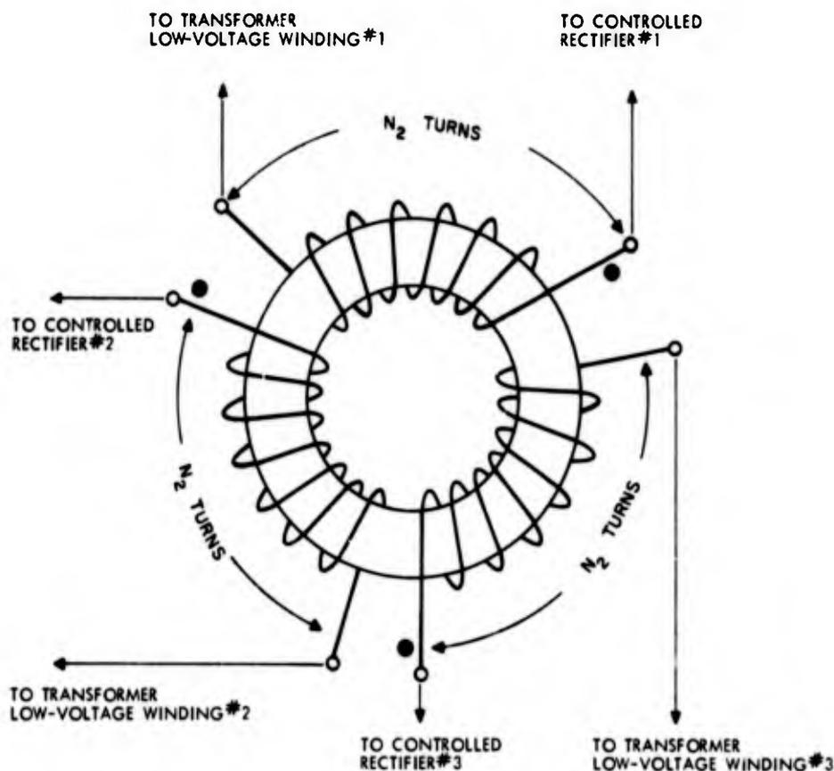
Fig. 4.3 Hold-Off Inductor Winding Configuration for 3 Parallel Discharge Paths
