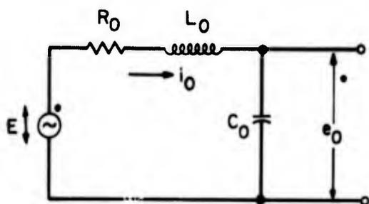
Fig. 3.10 Power-Supply Equivalent Circuit
