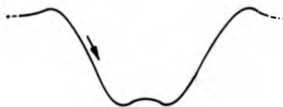
(F) HYPOTHETICAL REVERSE FLOW DOWN SIDE OF CAVITY FORMED BY BREAKING BUBBLE
