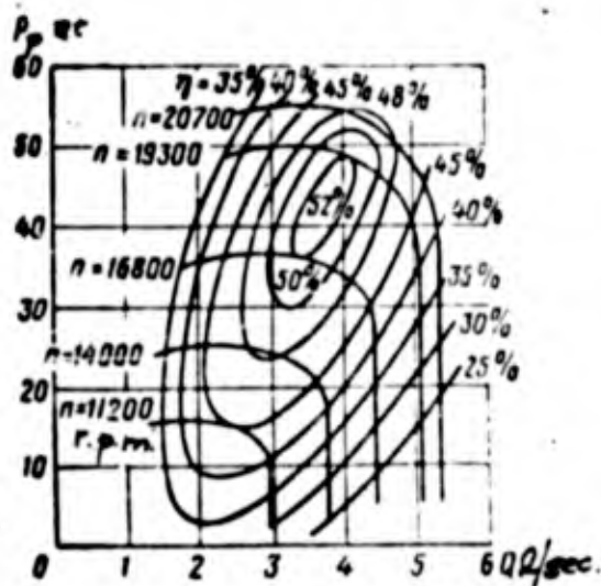
Figure 197. Characteristic of the centrifugal pump for nitric acid of engine R-3395, found in tests with water.
