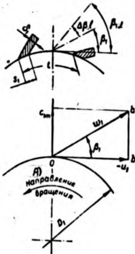
Figure 172. Diagram of velocities at the entrance to the wheel.
