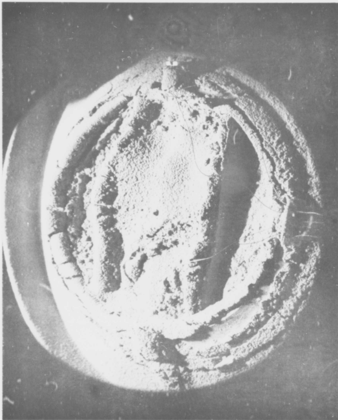
FIGURE V-3 BASALT POWDER SIEVED IN VACUUM AFTER DISRUPTION BY VIBRATION
