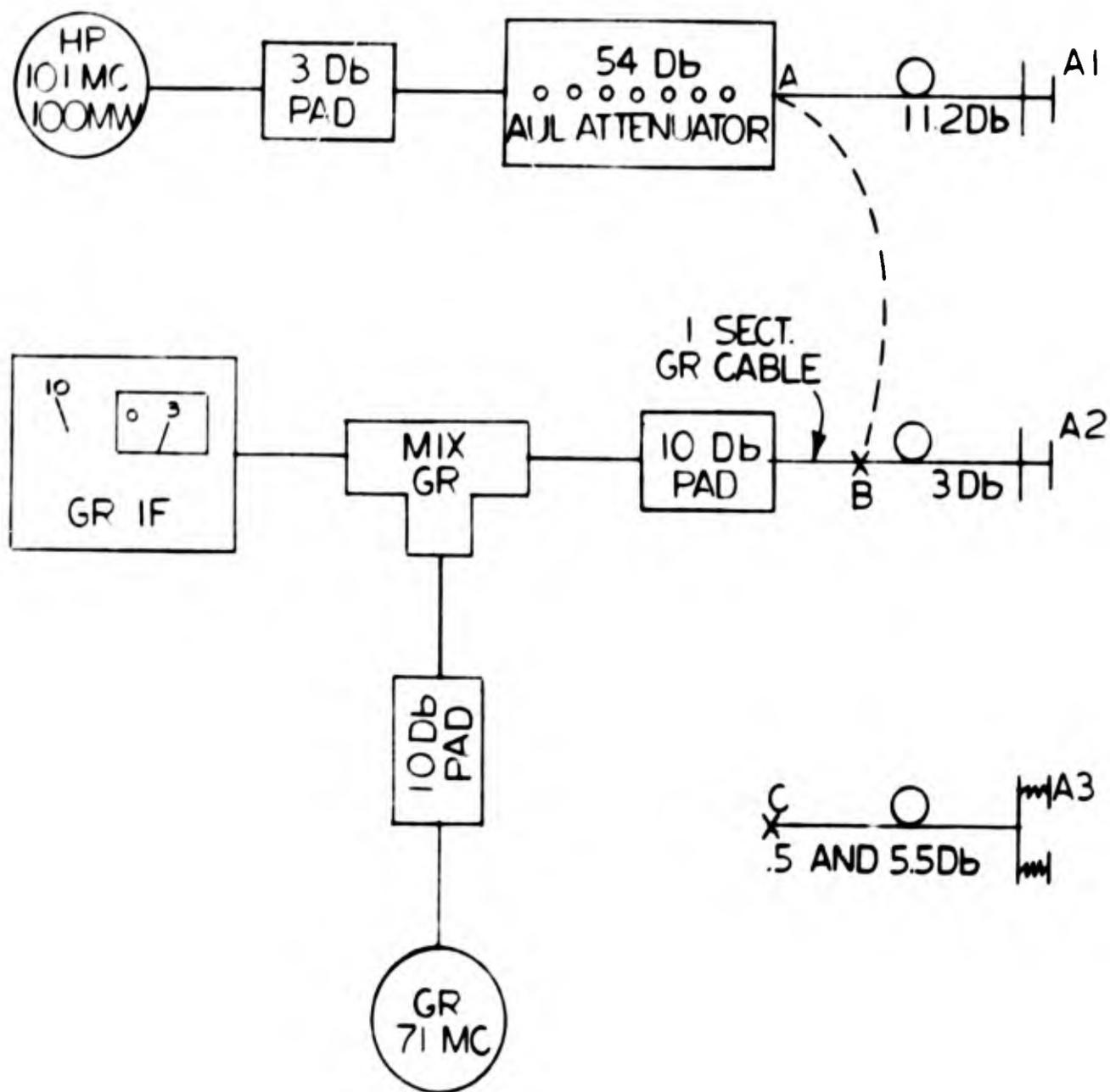
Figure 3-5. Test Set Up to Measure Transmission Loss
