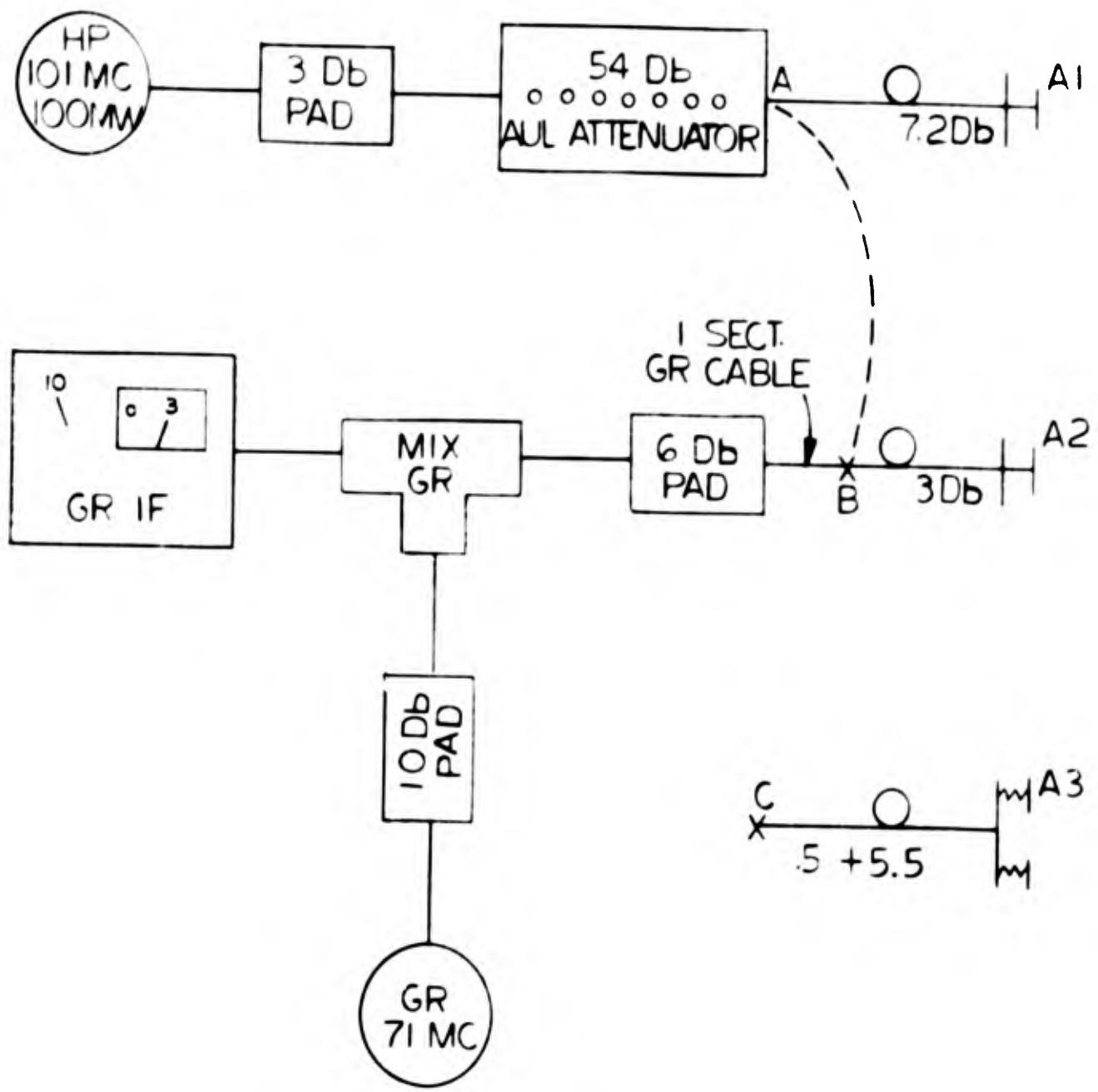
Figure 3-7. Test Set Up To Measure Transmission Loss
