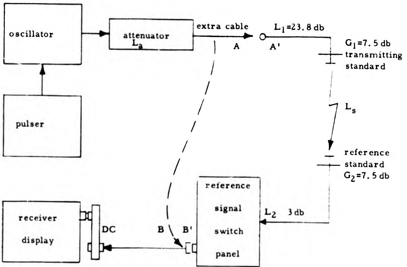
Figure 3-13. Test Setup for Path Loss Measurement
