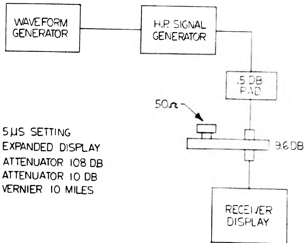
Figure 3-9. Display Calibration
