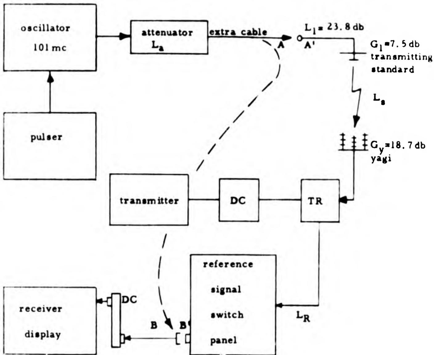
Figure 3-14. Test Setup for Receiver Line Loss Measurement
