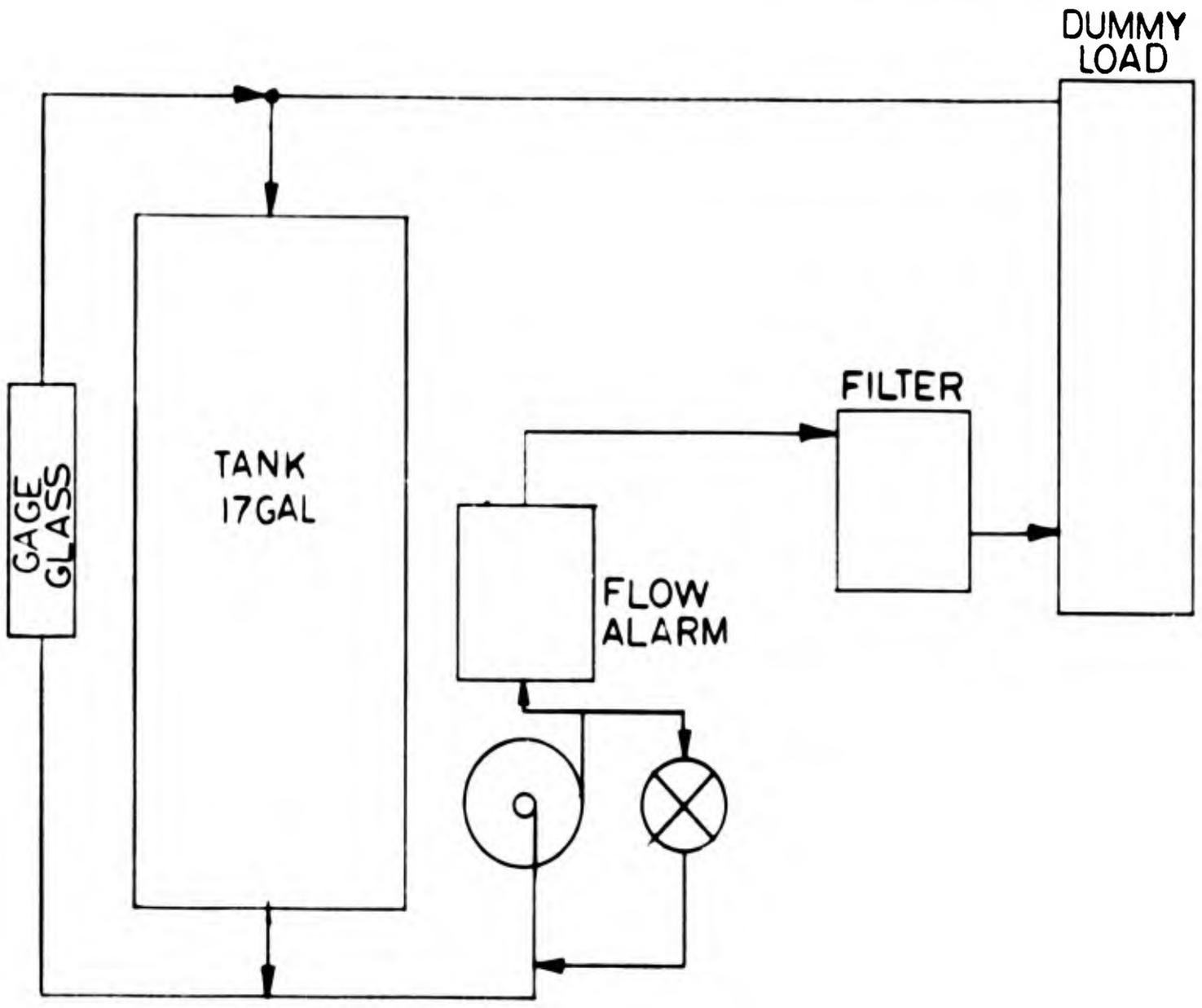
Figure 2-5. Coolant Flow Diagram
