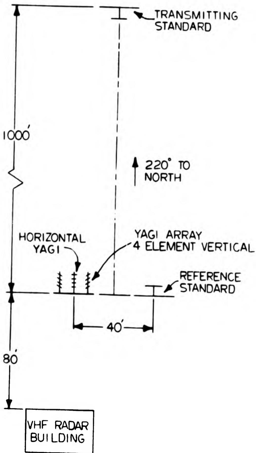
Figure 3-2. Calibration Antenna Layout
