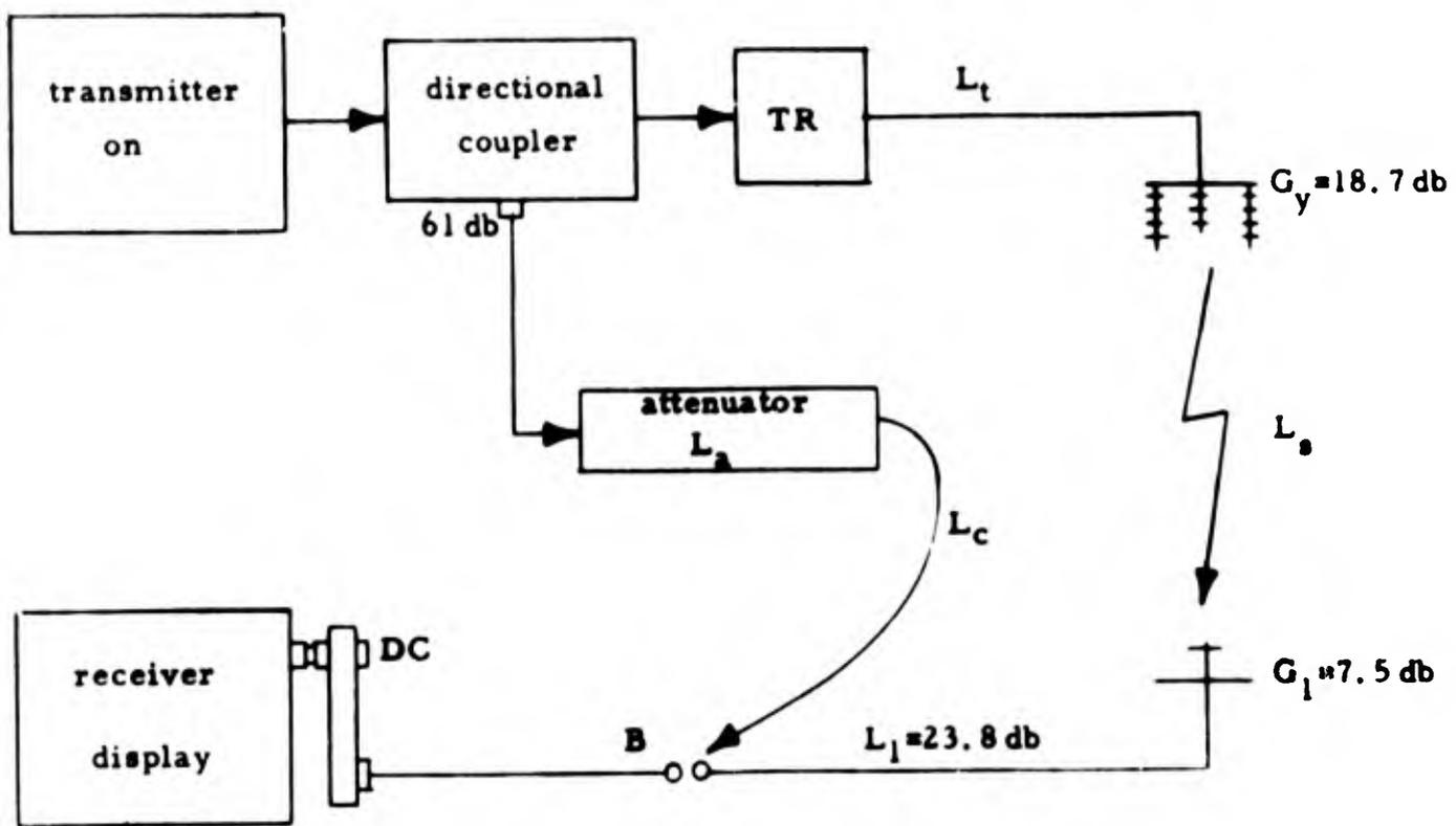
Figure 3-15. Test Setup for Transmitter Line Loss Measurement
