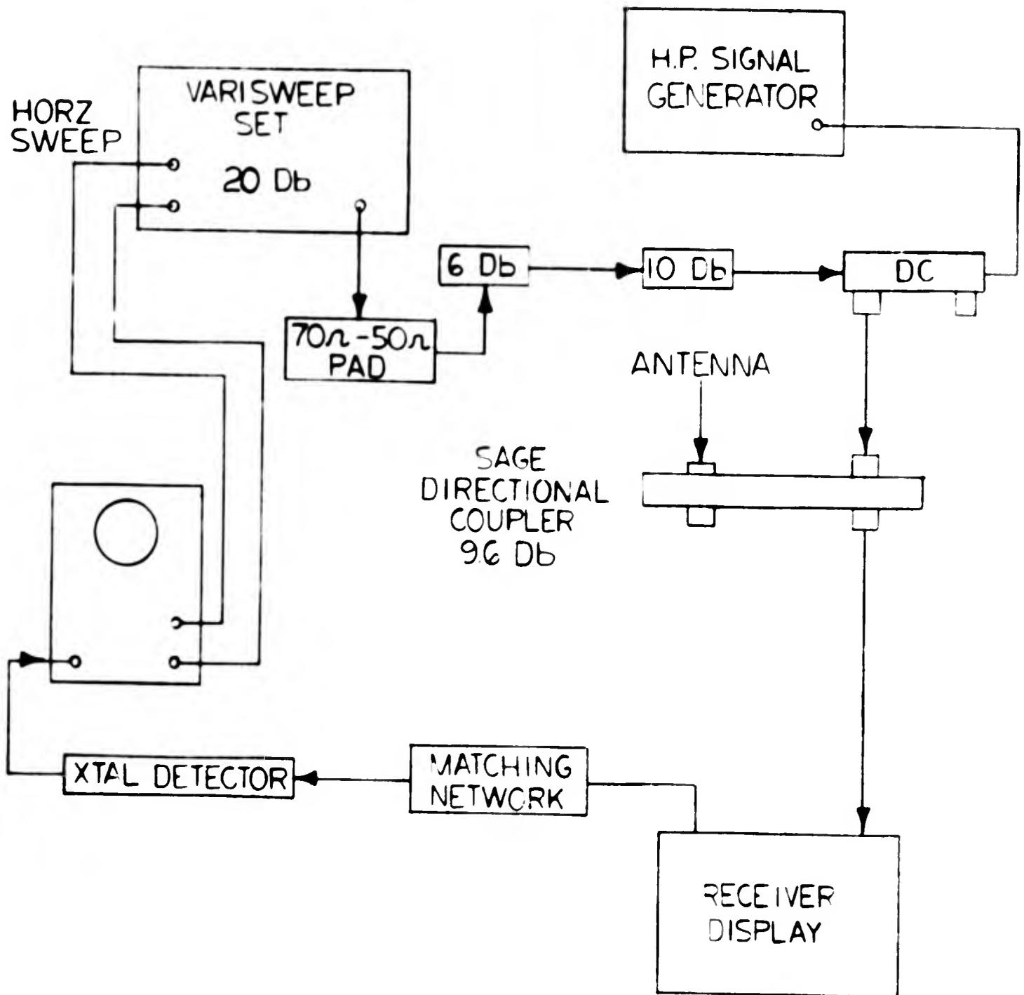
Figure 3-8. IF Bandwidth Measurement
