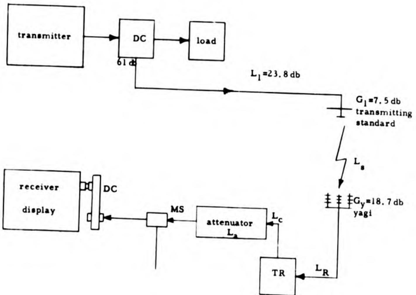
Figure 3-17. Test Setup for Second System Performance Verification
