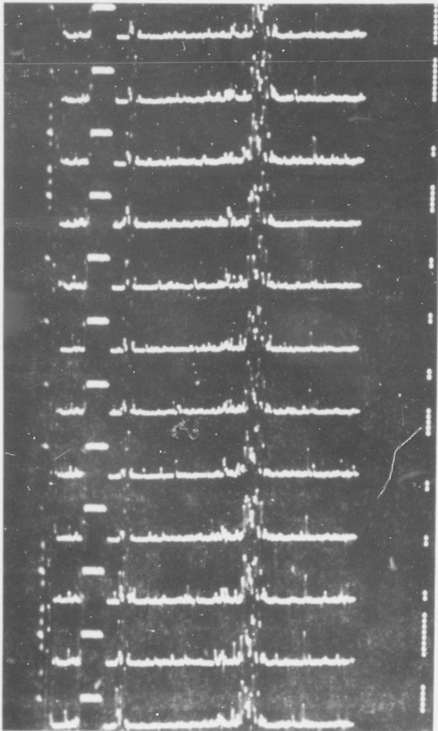
Figure 2-9. Continuous Recording of Vertically Polarized Signals Including Timing Marks. (1 MW peak power, 4 ms pulse vertical polarization, 100 NM sweep 155° Az, 0° el.)
