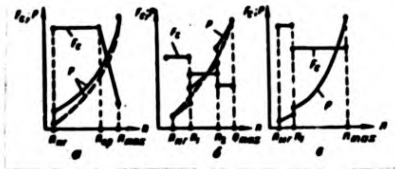
Fig. 220. Thrust P and nozzle throat area F_g as functions of rotor speed n with different control programs (the variation in thrust, following an optimum law, is shown by the dashed line). n_{cr} ) Rotor speed at cruising speed; n_{mg} and n_{max} ) rotor speed at low throttle setting and full throttle, respectively.
