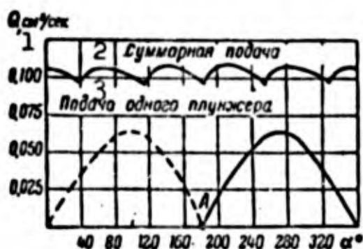
Fig. 203. Fuel feed rate Q as a function of pump-rotor angle of rotation \alpha . 1) Q , \text{cm}^3/\text{sec} ; 2) total feed rate; 3) feed rate due to one piston.
