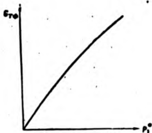
Fig. 294. Required characteristic for open-loop afterburner control system.
