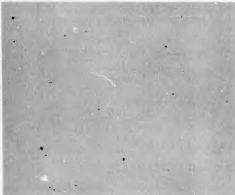
(b) Perpendicular to Rolling Direction 100X
