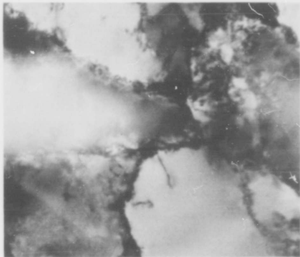
Fig. 32 - As-drawn tungsten wire, third area (40,000X).
