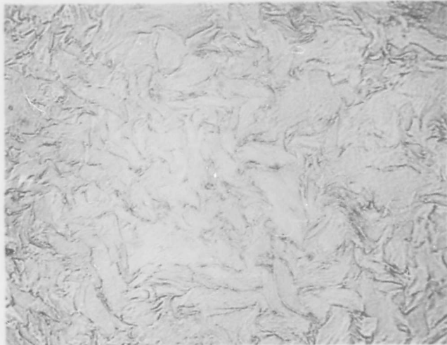
Fig. 68 - Columbium wire Cb-E1. Drawn 78.2% reduction in area, true strain 1.52. Transverse section (250X).
