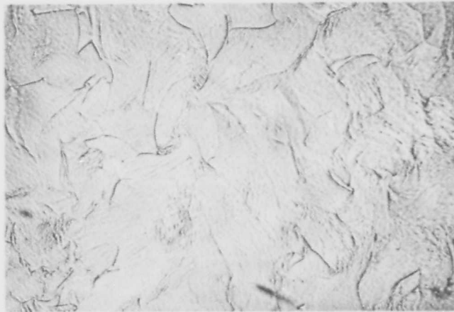
Fig. 67 - Columbium wire Cb-E1. Drawn 55.6% reduction in area, true strain 0.81. Transverse section (250X).
