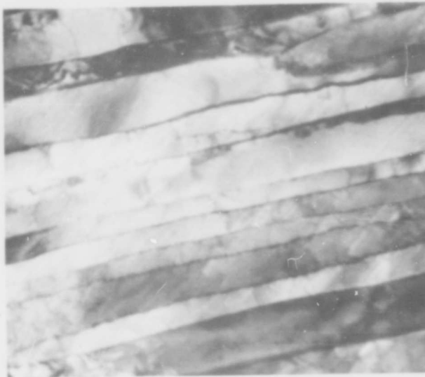
Fig. 44 - Tungsten wire annealed at 1000^{\circ}\text{C} for 10 min. (40,000X).
