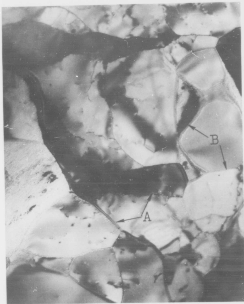
Fig. 16 - Thin-film electron micrograph of heavily worked and annealed (1 hour at 900°C) molybdenum (Mo-E1) strip, rolling plane section, showing clearly defined cell boundaries (arrow A) and cell coalescence (arrow B).
