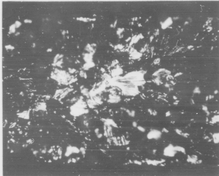
Fig. 23 - Light micrographs of high purity molybdenum (Mo-E1) strip, tensile specimen after testing at -70^{\circ}\text{C} , showing transgranular cleavage fracture. (a) Prepolished rolling plane section, rolling direction and tensile axis vertical, etched lightly after testing; note secondary cracks. (b) Fracture surface, note cleavage facets with river markings.
