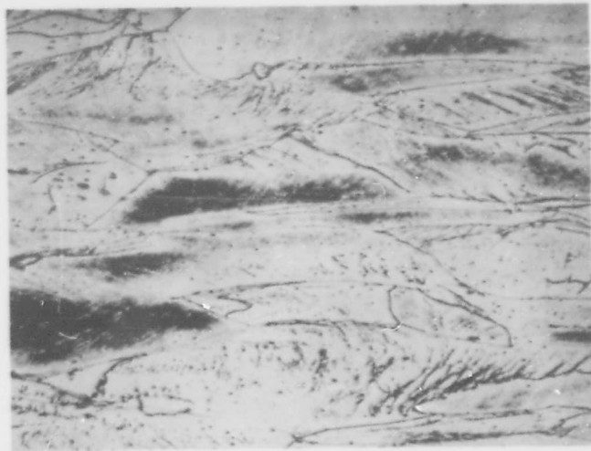
Fig. 55 - Fe-3.2% Si, drawn 66% reduction in area. Annealed at 500°C for 1 min. Fine scale substructure (dark) and diagonal subboundaries (315X).
