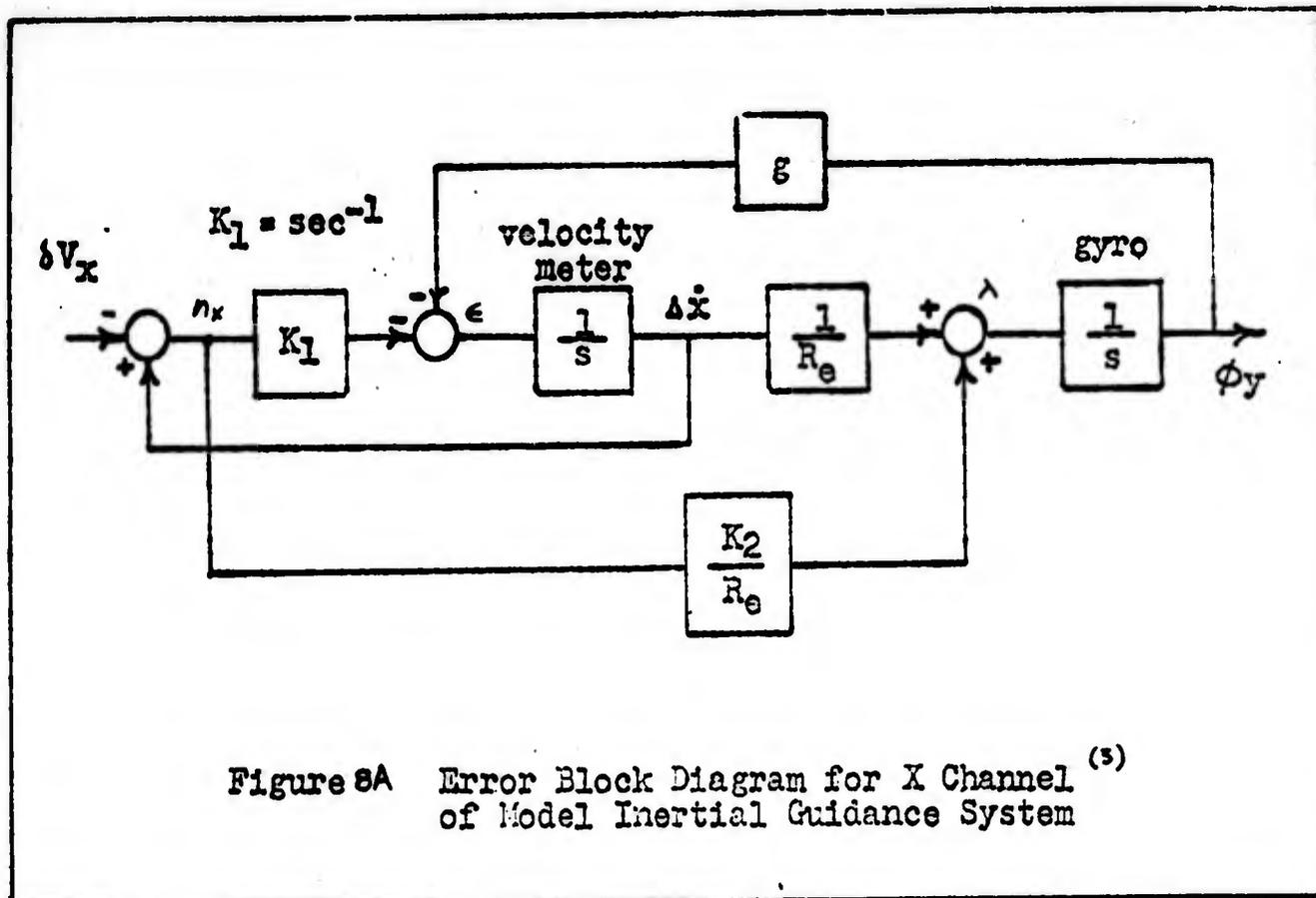
Figure 8A Error Block Diagram for X Channel<sup>(5)</sup> of Model Inertial Guidance System
