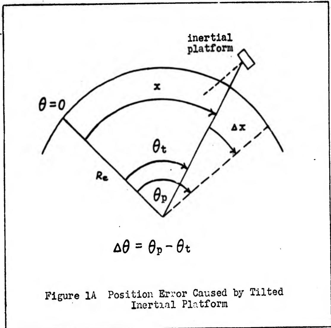
An accelerometer on the tilted inertial platform will measure the apparent acceleration,
