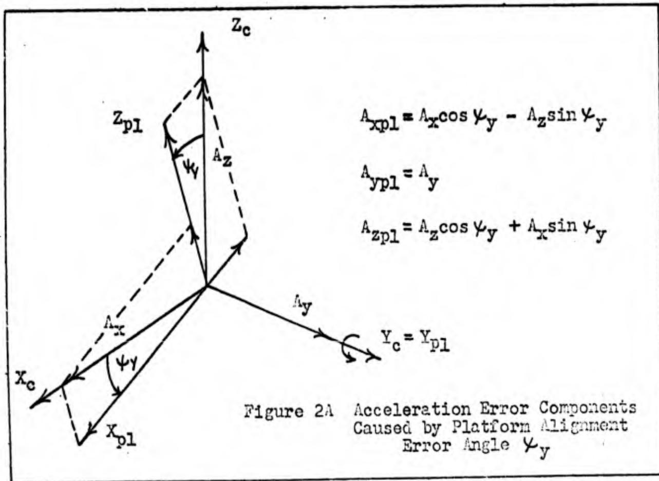
Introducing a component of platform angular error,  $\psi_y$ , and resolving the acceleration components to platform axes, produces acceleration error components in the (-)X and (+)Z directions, as shown in Figure 2A. In the figures, the subscript c indicates computer axes, t indicates true axes, and p1, p2, and p3 indicate successive positions of the platform axes.
