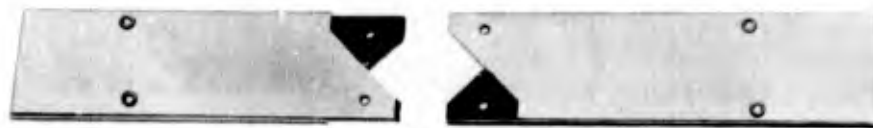
Fig. 3-2 Configuration of a typical mitered Tri-Plate junction.
