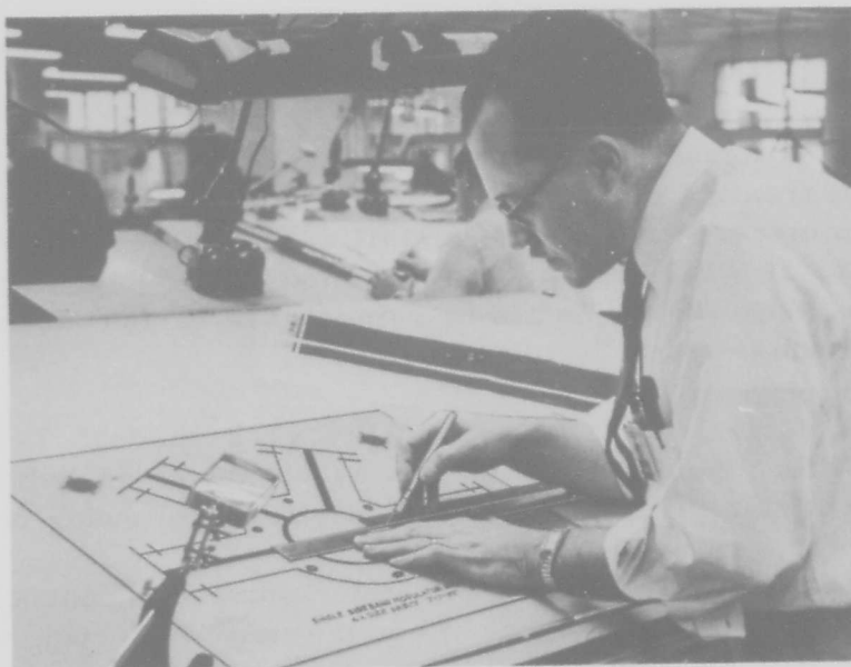
Fig. 7-8 Finishing touches on base-plate for S-band hybrid ring.
