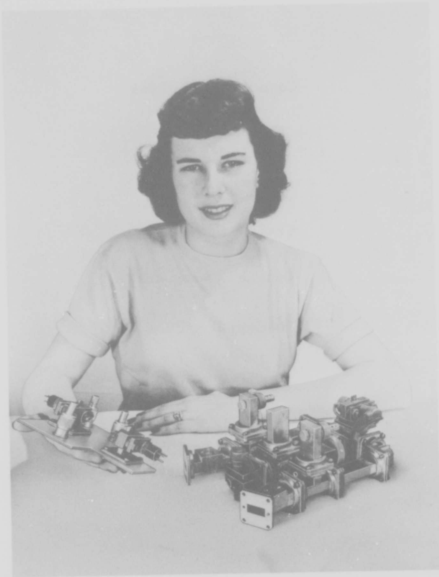
Comparison of Tri-Plate line and waveguide realizations of the same RF front end unit. The Tri-Plate line fabrication has one-eighth the weight and one-sixth the volume of its waveguide counterpart.
