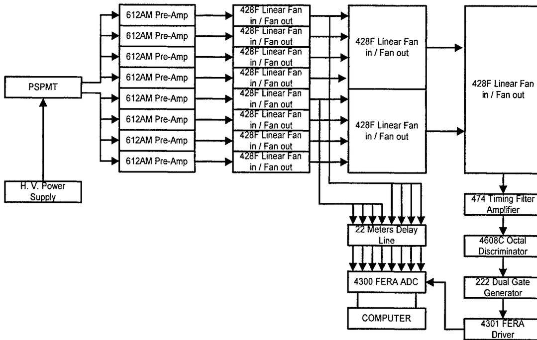
Figure 2. CAMAC modules used for data acquisition.
