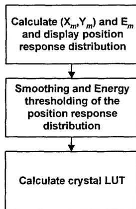
Figure 3. Flow diagram of the LUT generation algorithm
