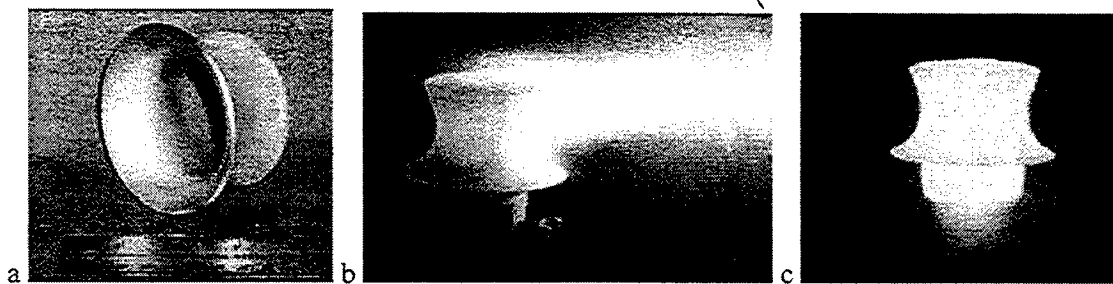
Figure 9: a). Non-eroding throat nozzles VPS fabricated at PPI. b) VPS fabrication to net shape. c) Same throat after nozzle material deposition.
