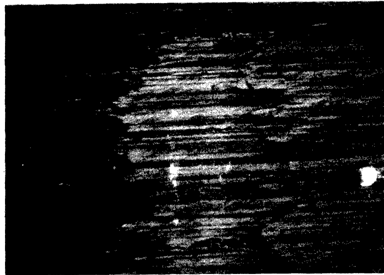
Figure 10. The grinding checks (arrows) in detail. Horizontal pattern is grinding grooves. Mag: 500x
