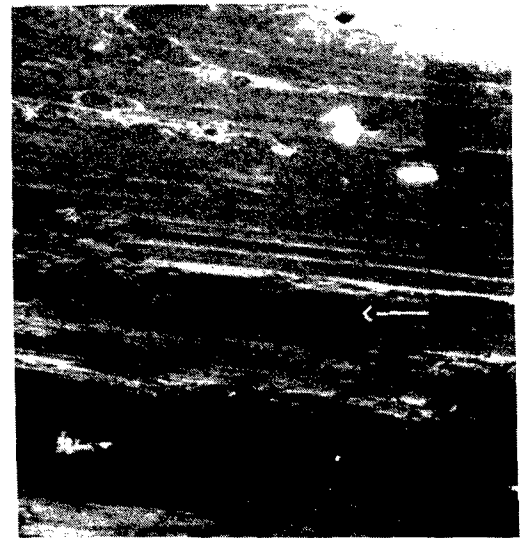
Figure 3. Crack (arrow) starting in machining groove. Mag: 85x
