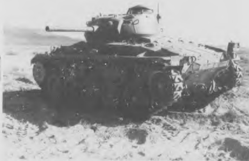
Tank - Before ↑ Looking Away From Zero Point After Looking toward Zero Point. Note: Tank ↓ fender in fore ground. Tank unserviceable due to broken lugs on tracks.
