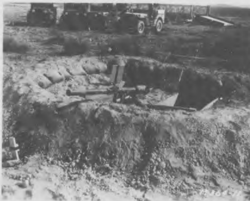
57 mm Recoilless Rifle - Before ↑ After Gun Blown 35 Yards Note: Burns ↓ on sand bags
