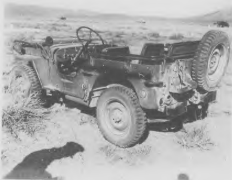
1/4 Ton Truck - Before ↑ After Moved 12 Yards to the rear ↓
