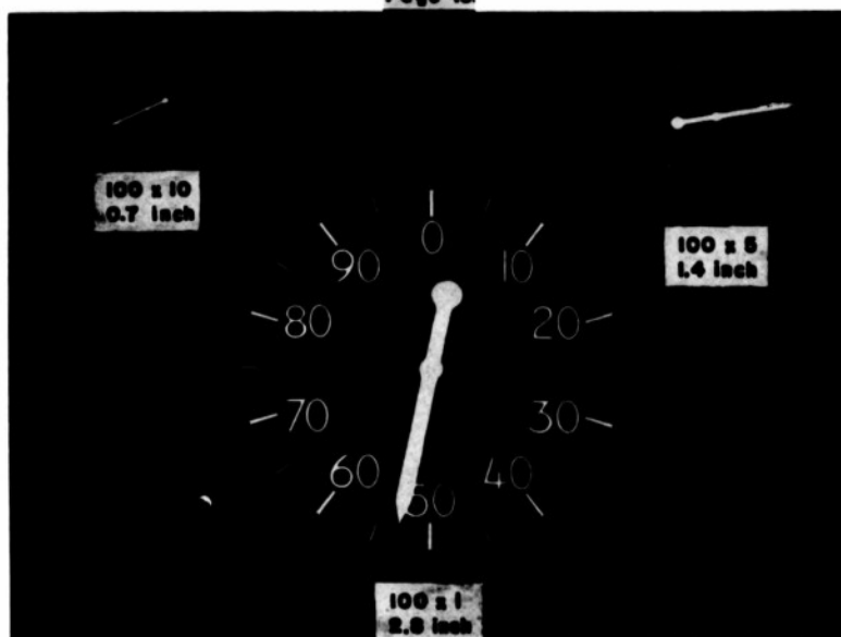
Figure 2. Dial designs and sizes used in the experiment. Each of the three designs shown were used in all three sizes indicated. The dimensions, in inches, given below are for the 2.8 inch dial. For the 1.4 inch and 0.7 inch dials all dimensions are respectively one half and one fourth as large.
