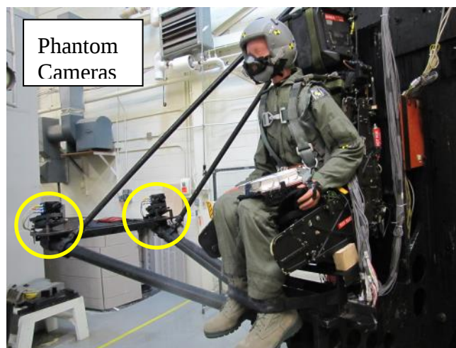
Figure 9. Phantom Miro-3 Cameras Mounted On-Board VDT Carriage
