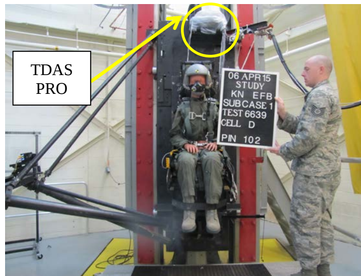
Figure 7. Location of TDAS PRO DAS System When Mounted on VDT Carriage
