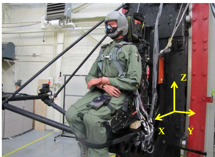
Figure 3. VDT Facility with Seat and Manikin Showing Impact Coordinate System
